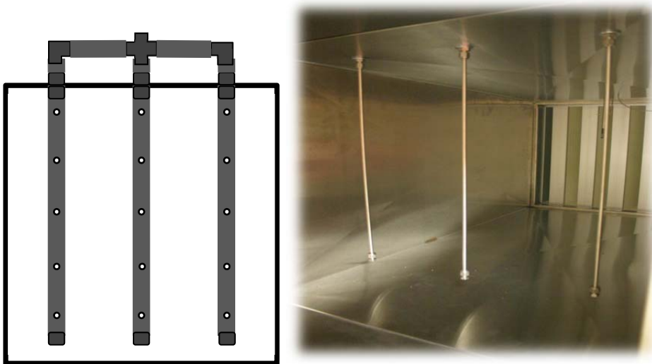
Figure 2.2. Ozone sampling grid used to measure ozone upstream and downstream of air cleaner
