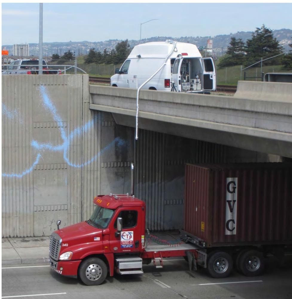
**Figure 2.** Instrumented van positioned on an overpass sampling the exhaust from a truck en route to the Port of Oakland.
