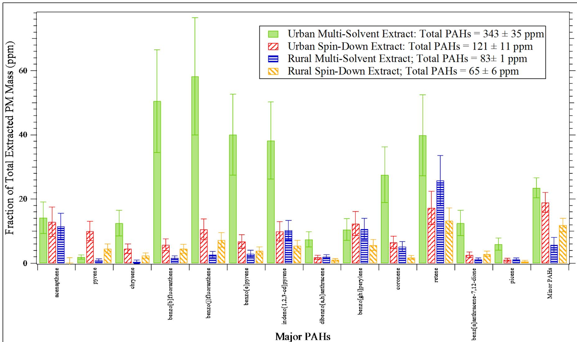
**Figure 4a.** Fraction of total extracted PM mass accounted for by major PAHs detected during TD-GCMS analysis of the urban and rural PM samples extracted via MSE and SDE; error bars represent 99% confidence intervals.
