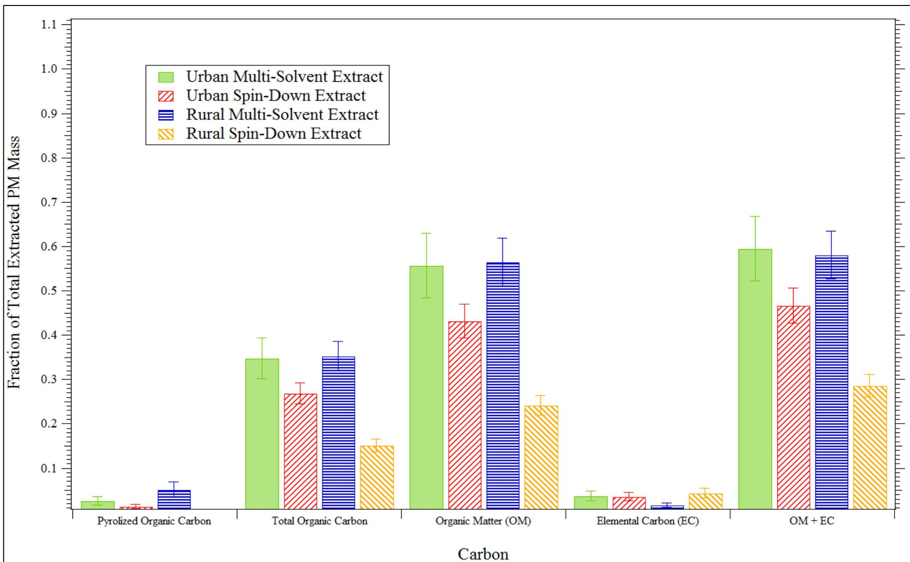
**Figure 6.** Fraction of total extracted PM mass accounted for by various carbon fractions determined from TOR measurements of the urban and rural PM samples extracted via MSE and SDE; error bars represent 99% confidence intervals.
