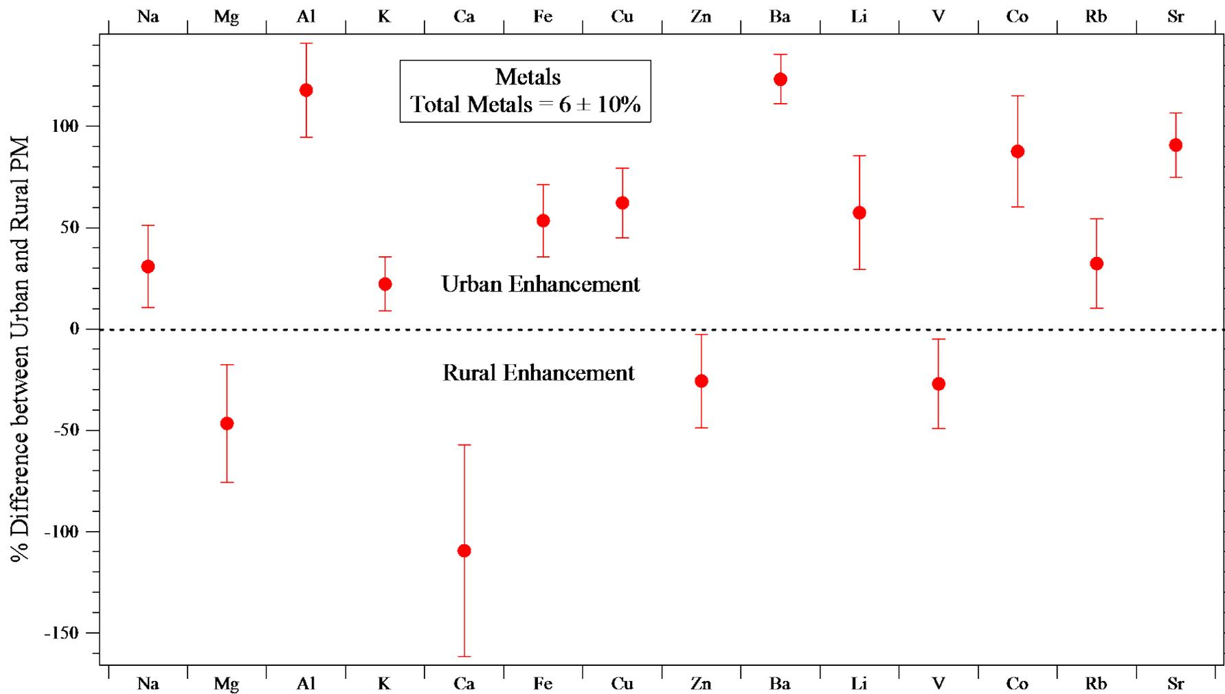
**Figure 9.** Percent difference between the urban and rural PM samples for trace metals determined via statistical analyses of ICP-MS data; see text for definition of percent difference used in this analysis. Only those metals showing statistically significant differences with p-values < 0.05 are included in the figure. The error bars represent 99% confidence intervals.
