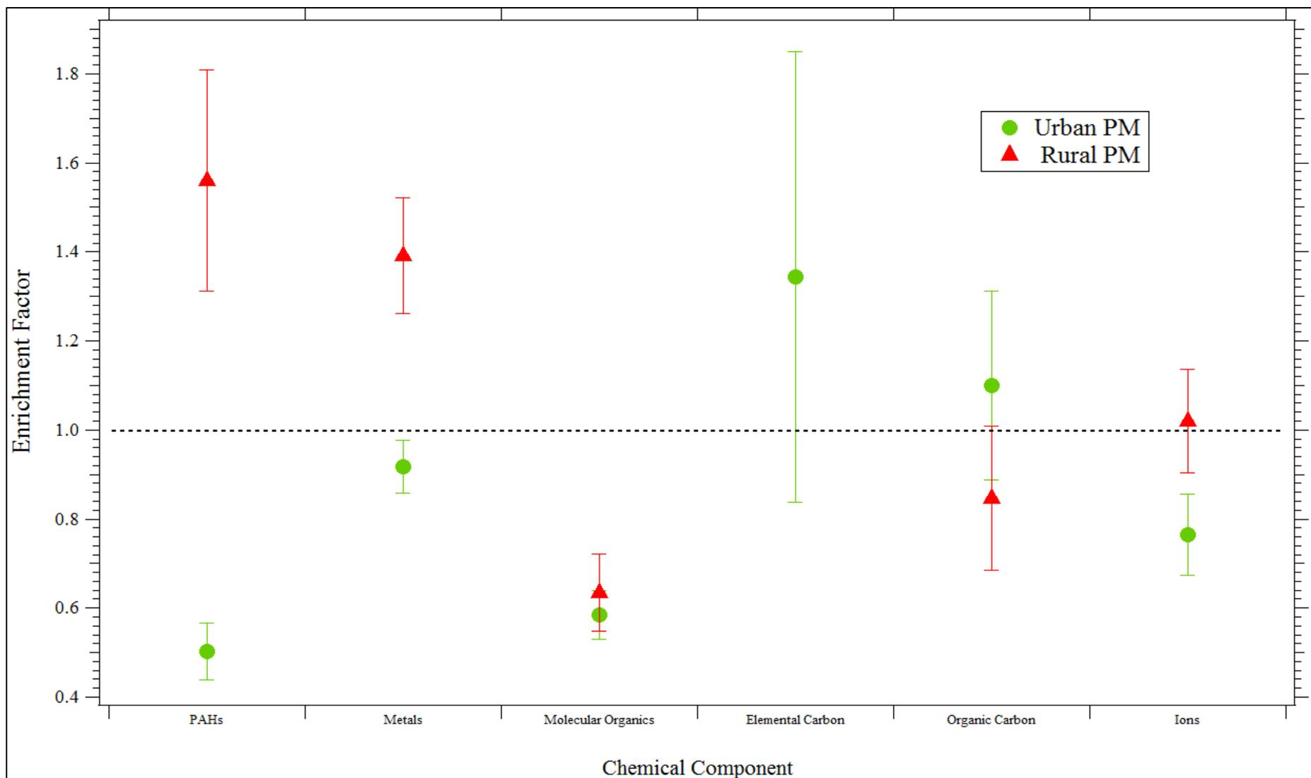
**Figure 8.** Enrichment factors for the various chemical components in the SDE extracted urban and rural PM samples relative to the MSE samples after adjusting the SDE data for the true mass of extracted PM; see text for discussion.
