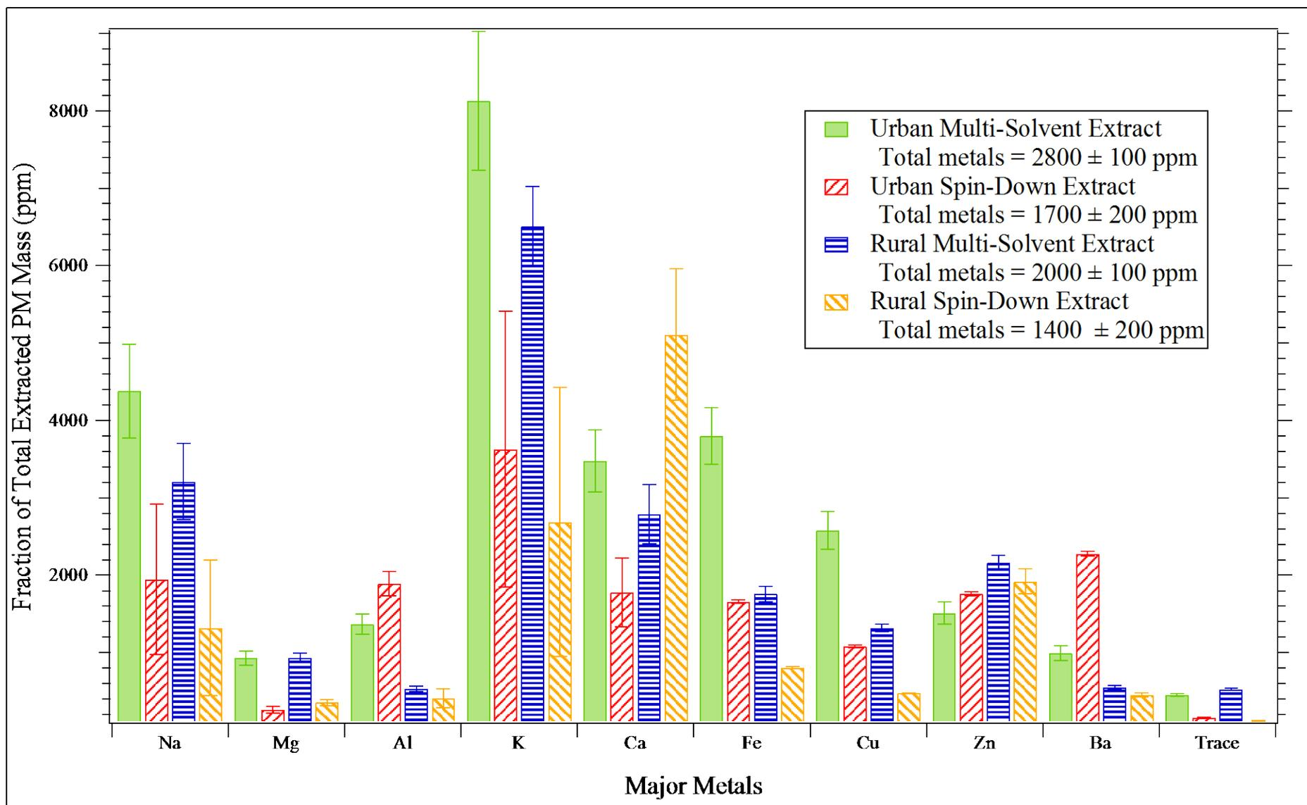
**Figure 2a.** Fraction of total extracted PM mass accounted for by major metals detected during ICP-MS analysis of the urban and rural PM samples extracted via MSE and SDE; error bars represent 99% confidence intervals.
