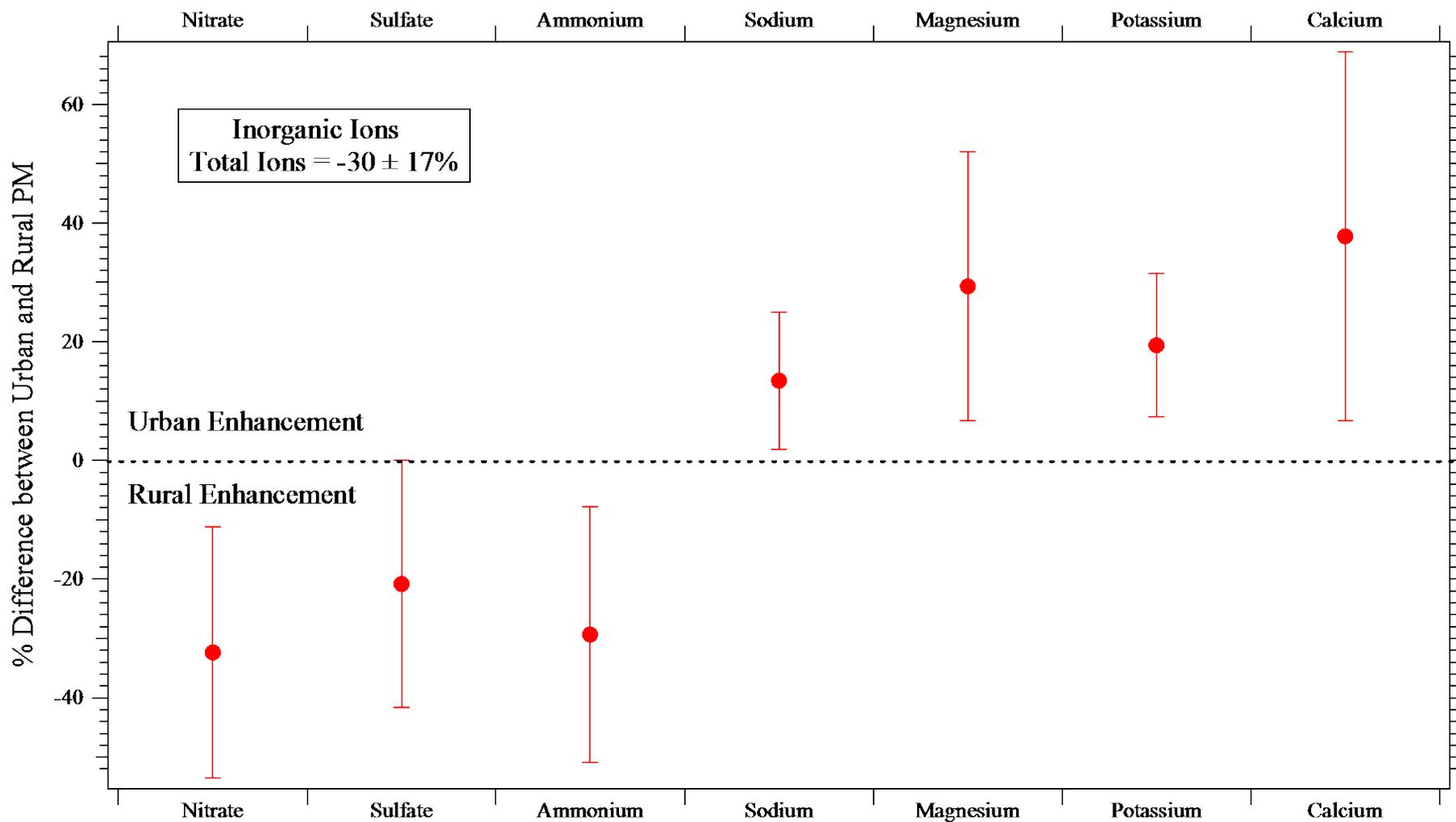
**Figure 11.** Percent difference between the urban and rural PM samples for inorganic ions determined via statistical analyses of IC, AC and AAS data; see text for definition of percent difference used in this analysis. Only those ions showing statistically significant differences with p-values < 0.05 are included in the figure. The error bars represent 99% confidence intervals.
