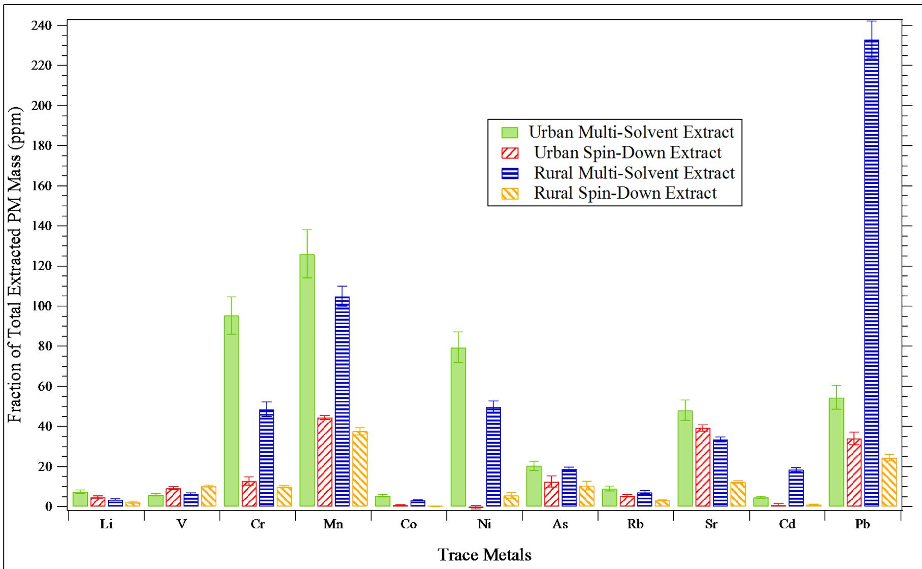
**Figure 2b.** Fraction of total extracted PM mass accounted for by trace metals detected during ICP-MS analysis of the urban and rural PM samples extracted via MSE and SDE; error bars represent 99% confidence intervals.
