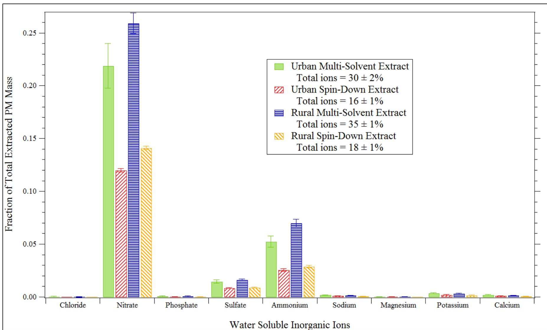
**Figure 3.** Fraction of total extracted PM mass accounted for by the water soluble inorganic ions detected during IC, AC and AAS analysis of the urban and rural PM samples extracted via MSE and SDE; error bars represent 99% confidence intervals.
