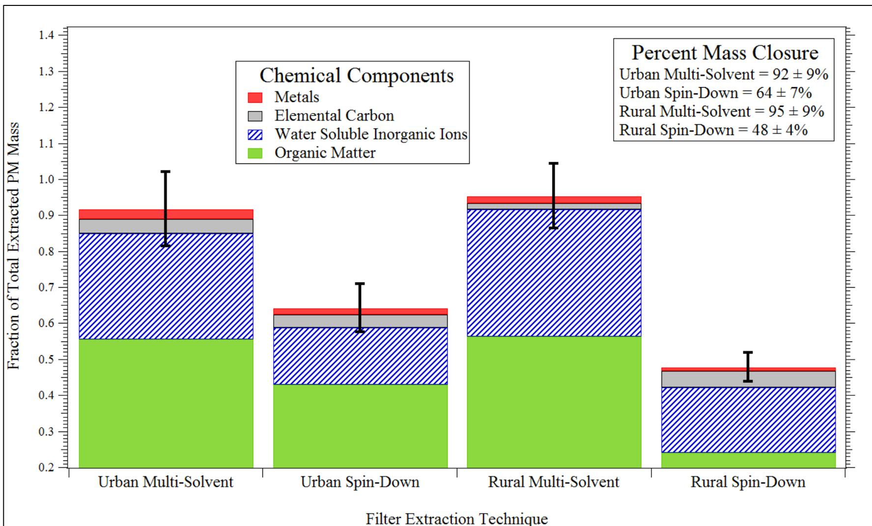
**Figure 7.** Fractional distribution of total extracted PM mass among the chemical components measured for the rural and urban PM samples extracted via MSE and SDE; error bars represent 99% confidence intervals for the component sum.
