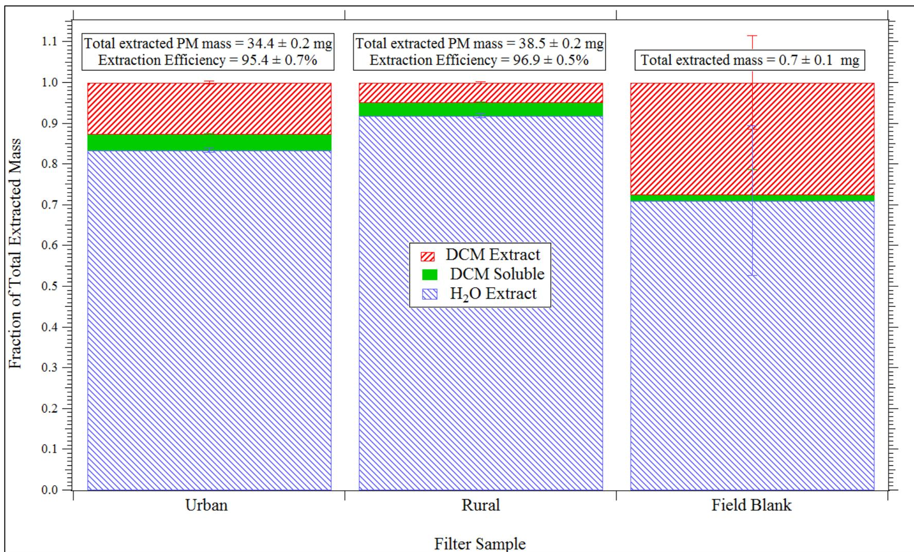
**Figure 1.** The fractional distribution of total extracted mass among the various steps of the multi-solvent extraction (MSE) for the urban, rural and field blank filter samples; see text for discussion.
