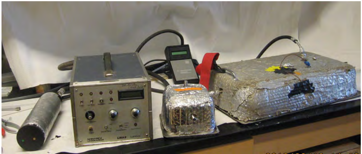
Figure 1A. Paraphernalia to measure NO x flux in the field. From left, vessel containing drying agent and Nafion™ tubing to remove air humidity, battery-powered Scintrex (LMA-3) NO x analyzer, chamber used in alfalfa fields, chamber used in corn, tomato, and wheat systems.
