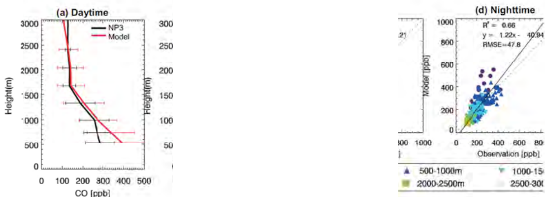
Figure 5.4: Simulated and observed concentrations of CO vertical profiles for the ensemble of CalNex flights during a) daytimes and b) nighttimes. The horizontal bars indicate the standard deviations. Also shown are the scatter plots (c-d), with values at different altitudes color-coded.
