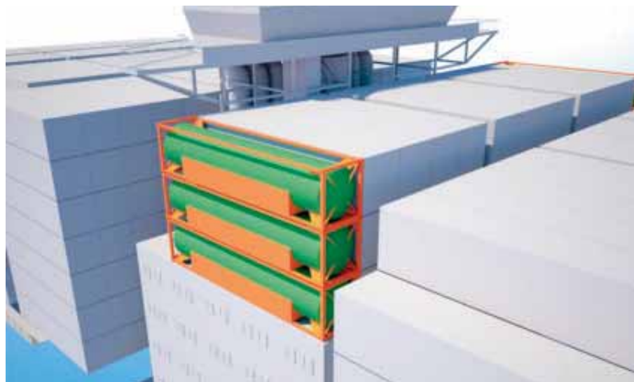
■ Fig. 8 – Containerized LNG storage tanks located outdoors on top of the deckhouse.
