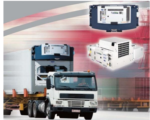
Figure 9. Diesel generator set mounted on an intermodal RSC
