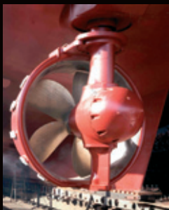
Wärtsilä modular steerable thruster.
