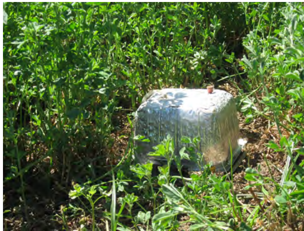
Figure 11A. Chamber base and chamber used in alfalfa systems.
