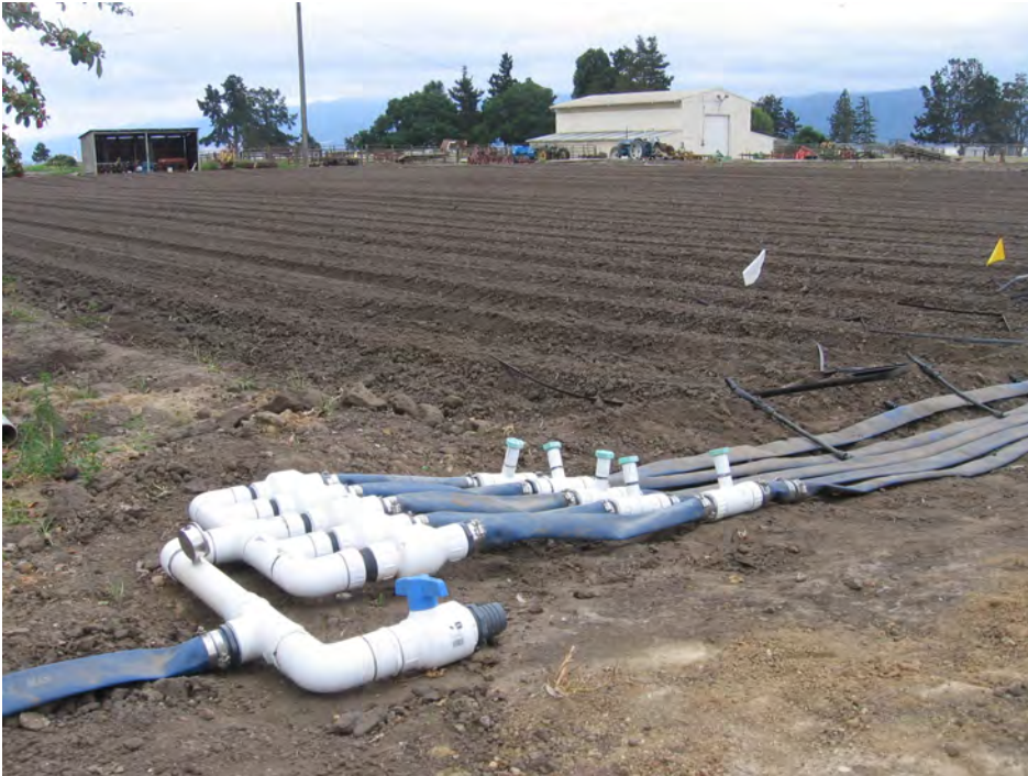
Figure 5A. Irrigation manifold with five ports used to inject fertilizer during irrigation (fertigation) at the Hartnell College Ranch, Salinas, where the lettuce crop was fertilized at five different N rates.
