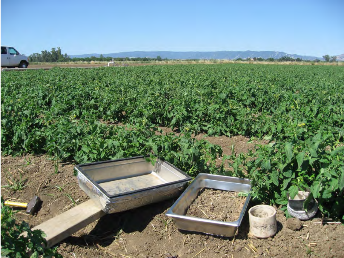
Figure 9A. Rectangular chamber base and chamber used in tomato and lettuce systems on the beds, and round chamber base and chamber used in the furrows of those systems.
