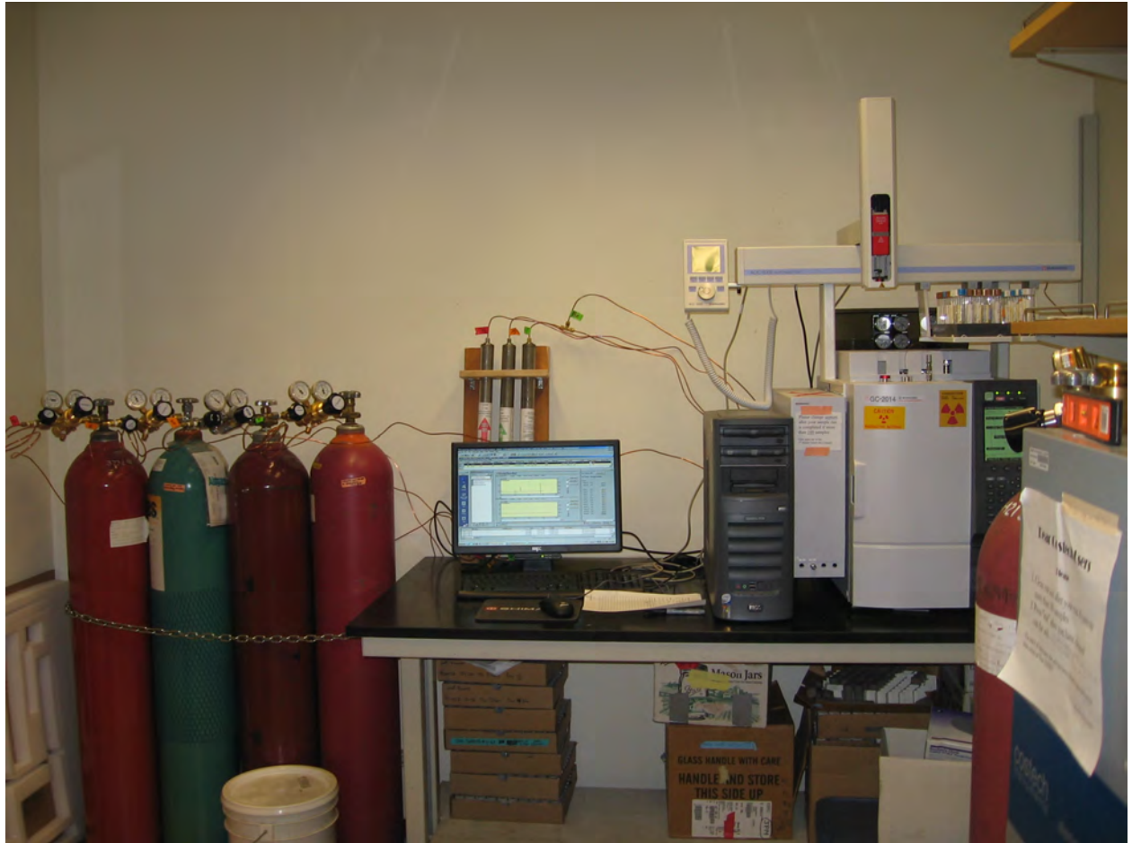
Figure 2A. Gas chromatograph with autosampler in Dr. Horwath's laboratory.
