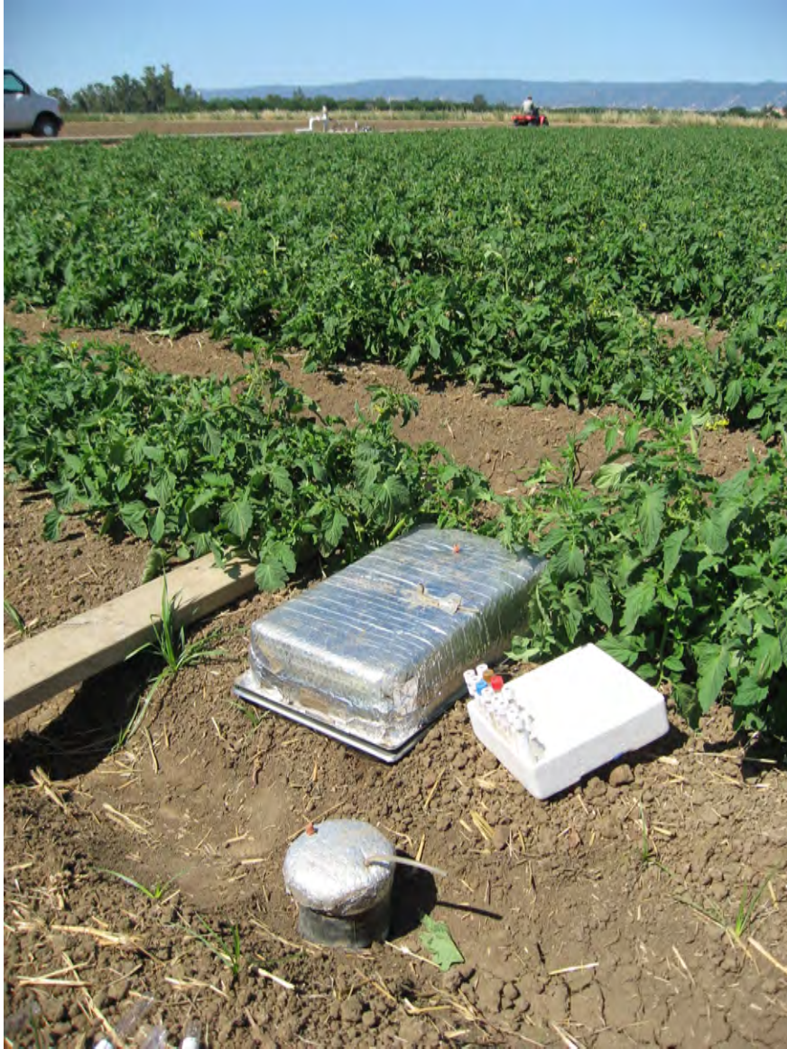
Figure 10A. Bed and furrow chambers closed during flux measurements.
