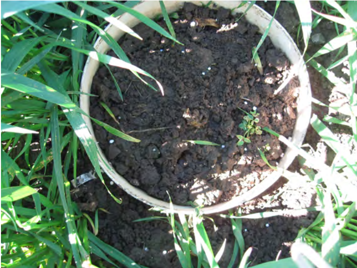
Figure 8A. Round PVC chamber base used in the wheat and rice systems.
