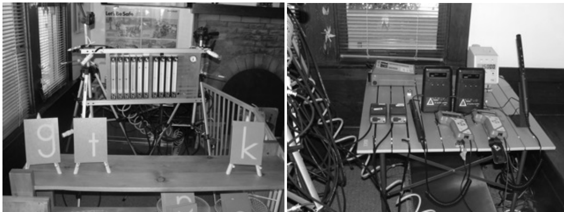
Figure 2. Indoor equipment set-up at an ECE facility. Left image includes the flowmeters and integrated samplers. Right image shows real-time devices.
