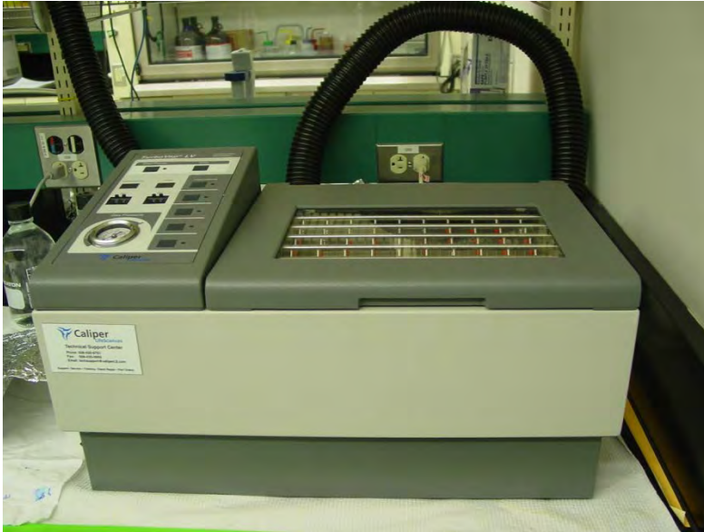
Figure 3. Turbo Vap LV with a custom made tray to hold 60 ml vials prepared by the EPA machine shop.
