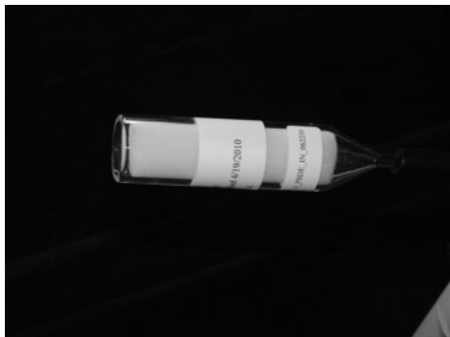
Figure 3. PUF cartridge used to sample SVOCs with corresponding sample label affixed to cartridge.
