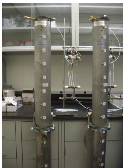
Plate 2.2.1. Photograph of soil columns used for shank injection studies.
