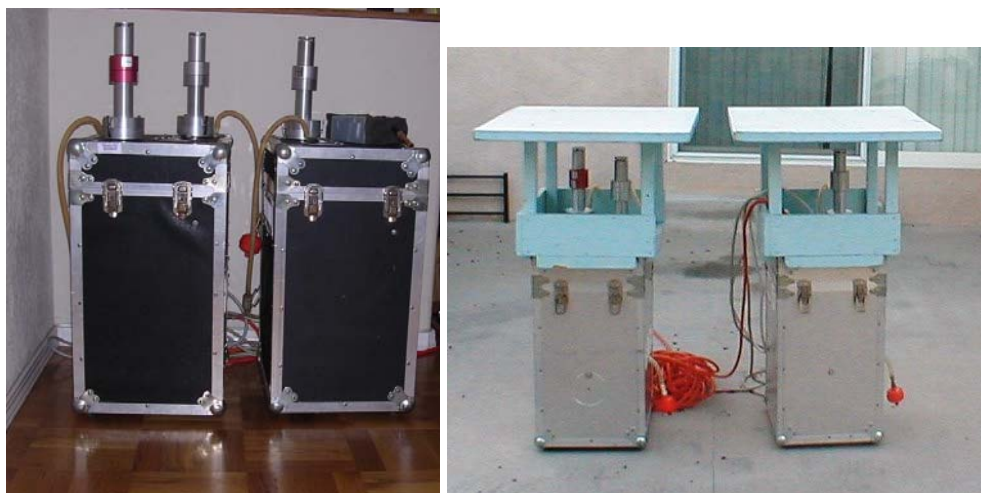
Figure 2. Indoor and outdoor home monitoring. Harvard impactor samplers (Air Diagnostics and Engineering, Inc., Naples, ME).
