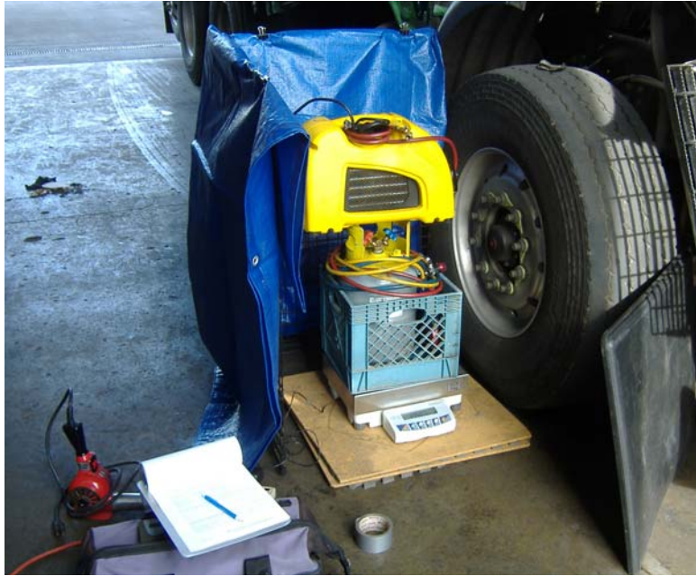
Figure 3. Recovery System Being Weighed after a Recovery
