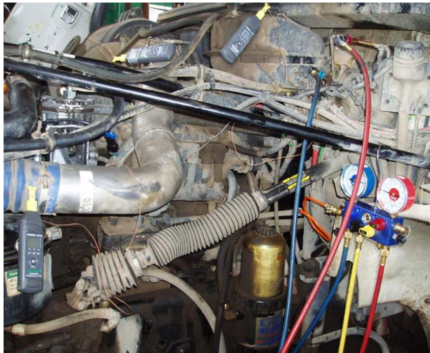
Figure 2. Manifold and Thermocouples during a Recovery
