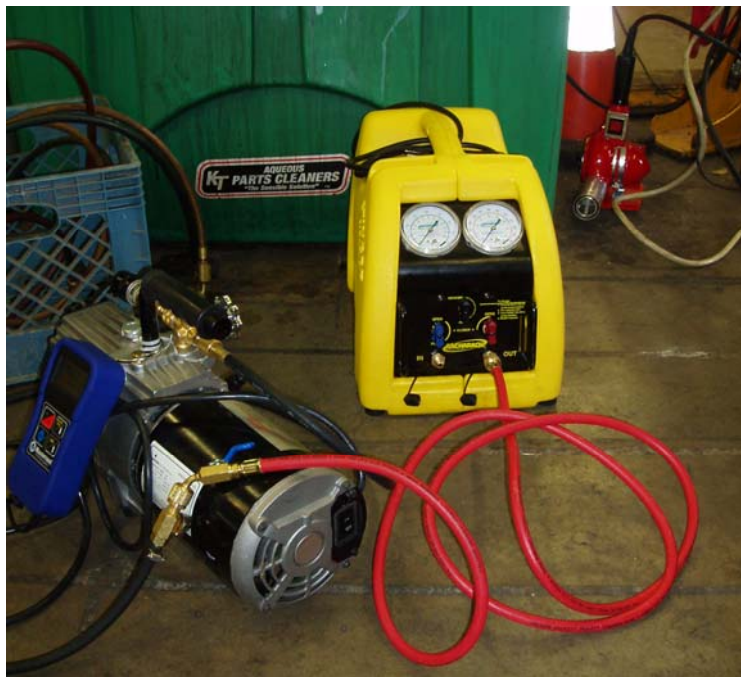
Figure 1. Evacuation of the Recovery Unit and Hose before a Test
