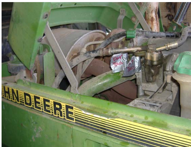
Figure 5. Anti-tamper Measures to Discourage MAC Service during a Test
