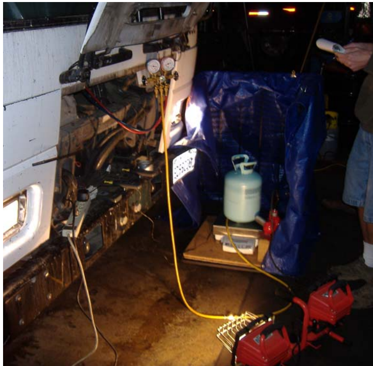
Figure 4. Recharging a MAC after all R134a was Removed
