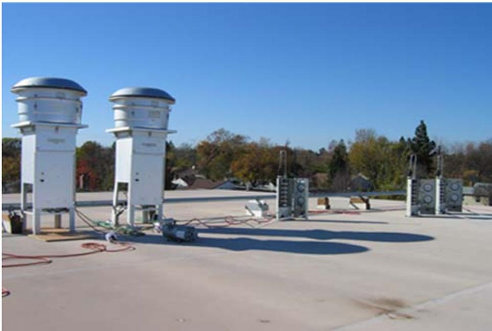
Figure 5. MOUDI and PM<sub>10</sub> samplers installed on the rooftop of a school gymnasium.
