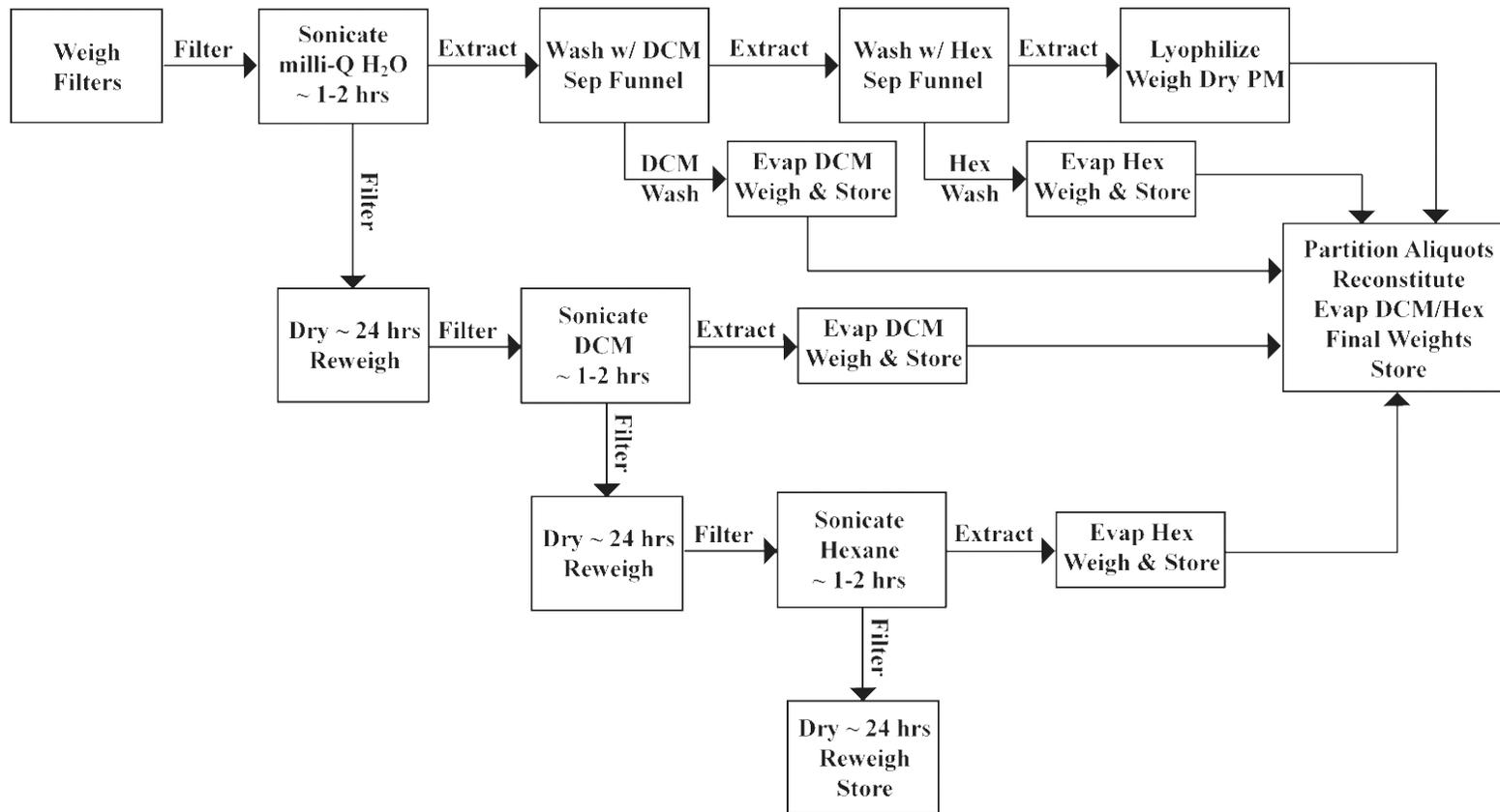
**Fig 3-1.** Flow diagram of the filter extraction and particle reconstitution process for Teflon coated borosilicate glass fiber afterfilters.
