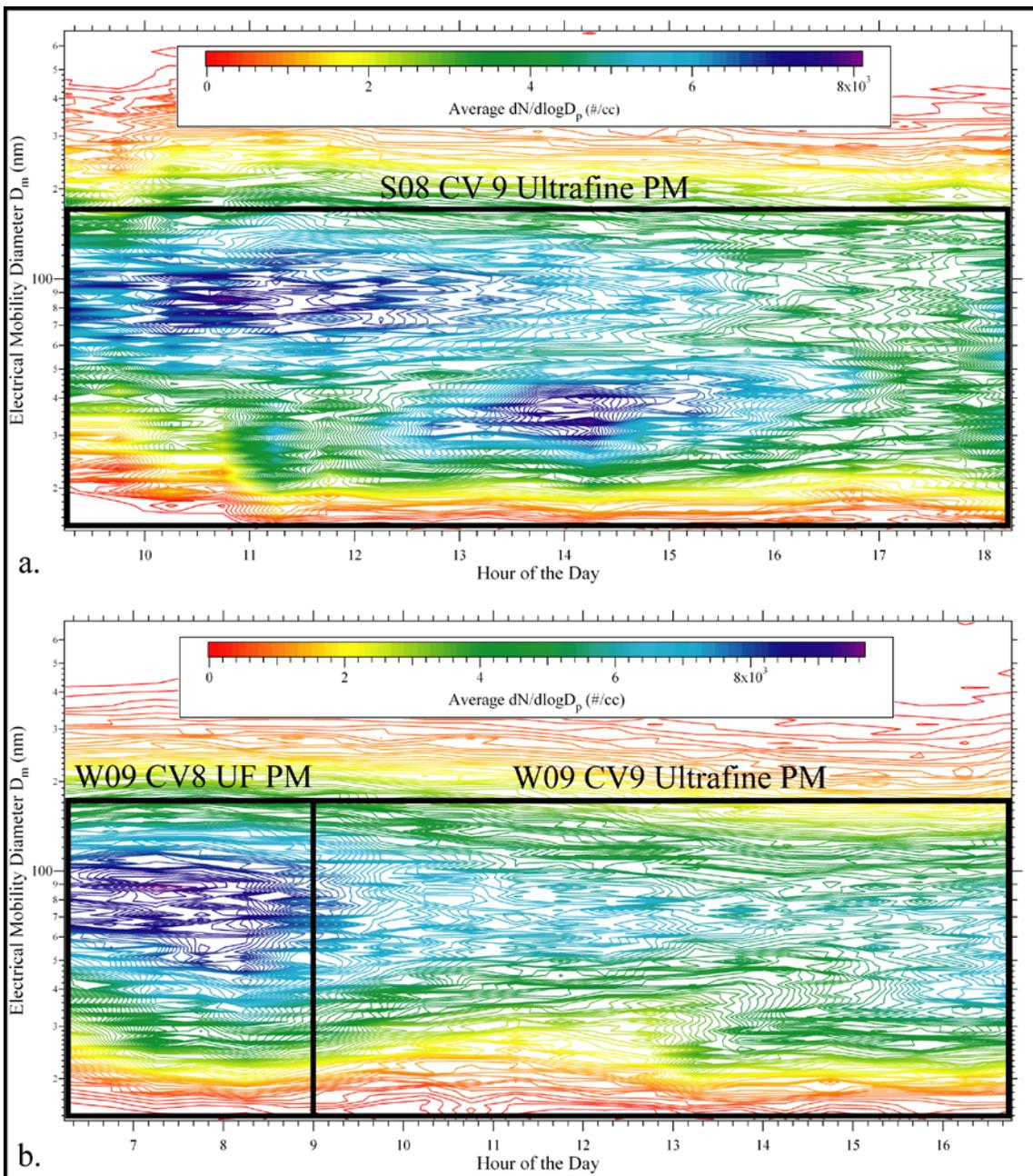
**Figure 4.1.** Contour plots showing the study average daytime particle number distribution for the (a) summer 2008 and (b) winter 2009 experiments. The time periods corresponding to the various timed ChemVols are outlined and labeled in the figures; see text for details.
