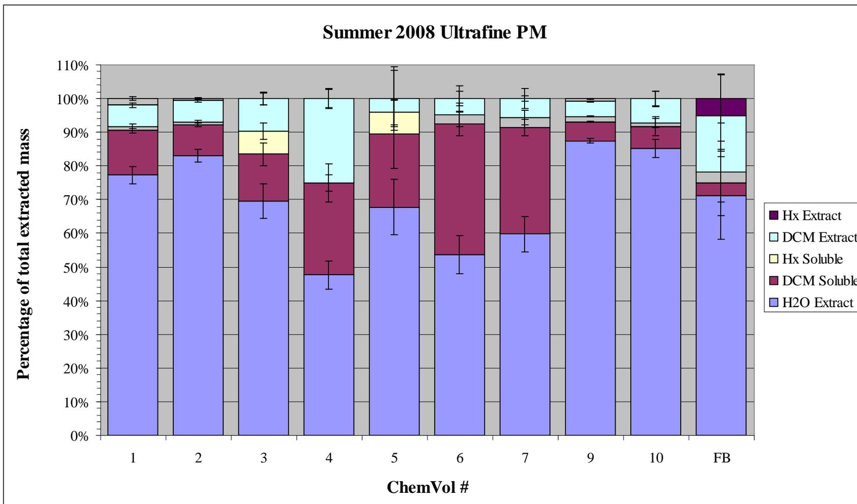
**Figure 3-3.** The fractional distribution of total extracted mass among the PM components removed during the various steps of the filter extraction process for the ultrafine PM fractions collected during the summer 2008 experiment by ChemVol; FB = field blank. See text for a description of the various PM components.
