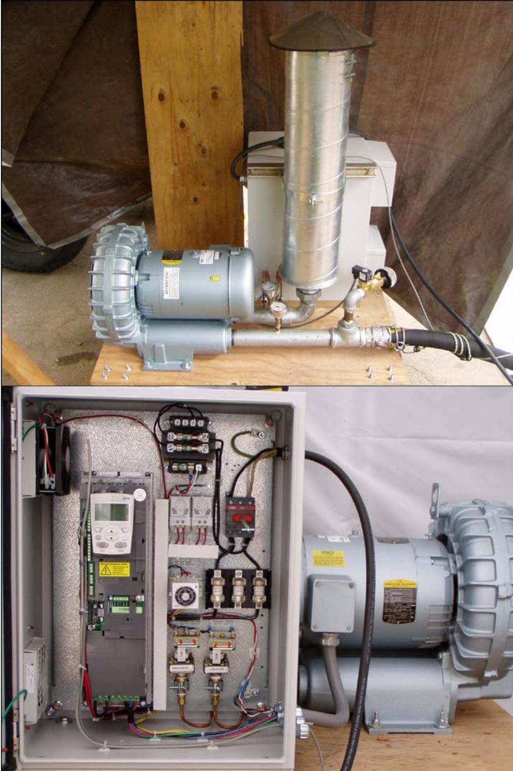
**Figure 2S-6.** Picture of the blower assembly (top) and variable frequency AC drive (bottom). See text for description.
