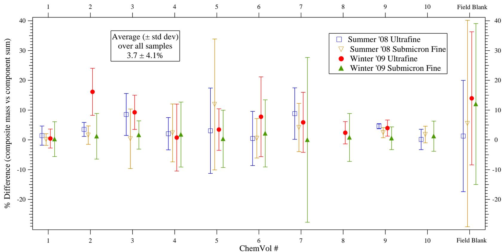
**Figure 3-7.** Percent difference between the total extracted mass obtained by weighing the final reconstituted composite extracts versus summing the component masses obtained during the various steps of the filter extraction process; see text for a description of the filter extraction process and associated PM components.
