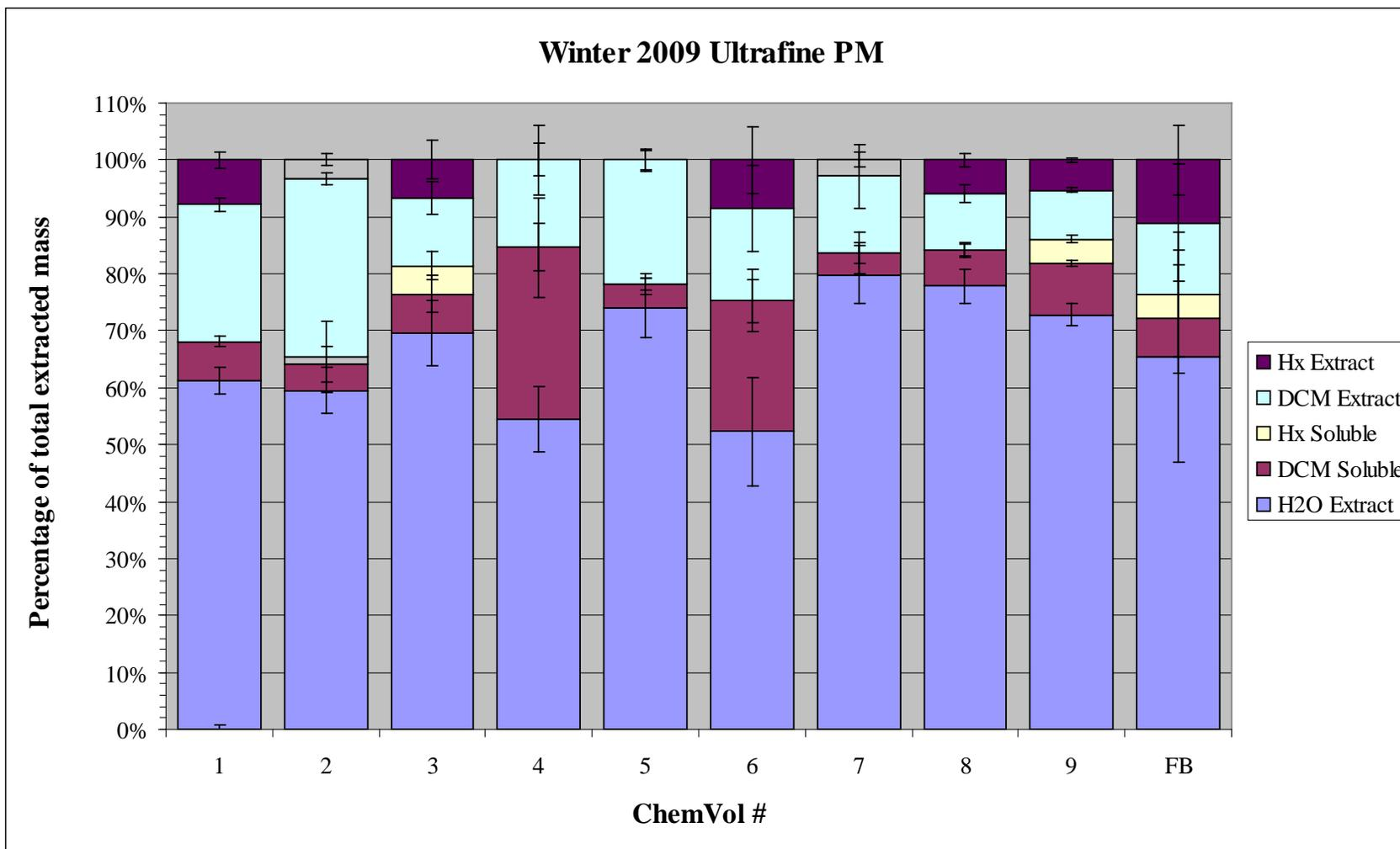
**Figure 3-4.** The fractional distribution of total extracted mass among the PM components removed during the various steps of the filter extraction process for the ultrafine PM fractions collected during the winter 2009 experiment by ChemVol; FB = field blank. See text for a description of the various PM components.
