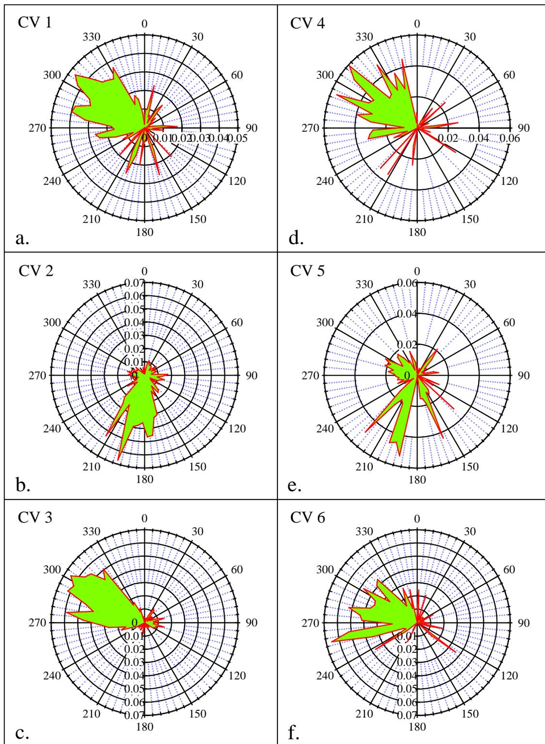
**Figure 4.4.** Wind direction frequency distributions for the source-oriented ChemVols during the winter 2009 experiment; see text for a discussion of these plots.
