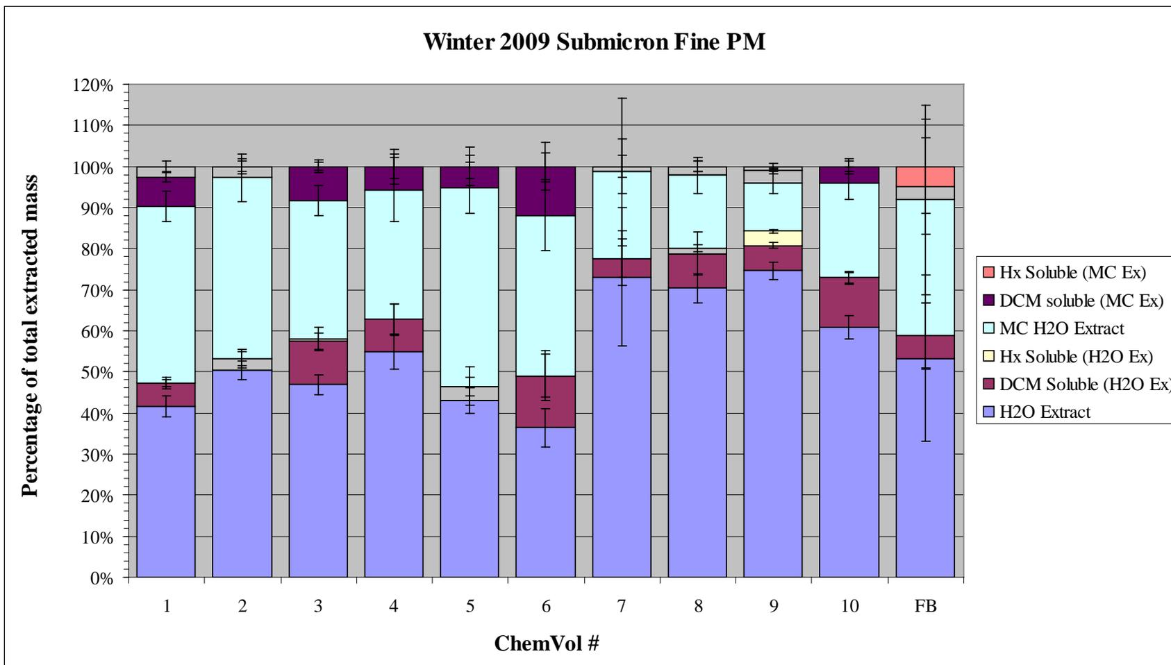
**Figure 3-6.** The fractional distribution of total extracted mass among the PM components removed during the various steps of the filter extraction process for the ultrafine PM fractions collected during the winter 2009 experiment by ChemVol; FB = field blank. See text for a description of the various PM components.
