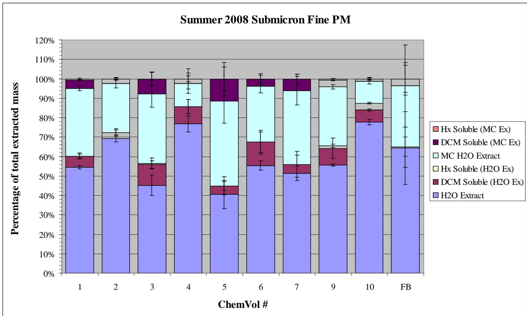
**Figure 3-5.** The fractional distribution of total extracted mass among the PM components removed during the various steps of the filter extraction process for the ultrafine PM fractions collected during the summer 2008 experiment by ChemVol; FB = field blank. See text for a description of the various PM components.
