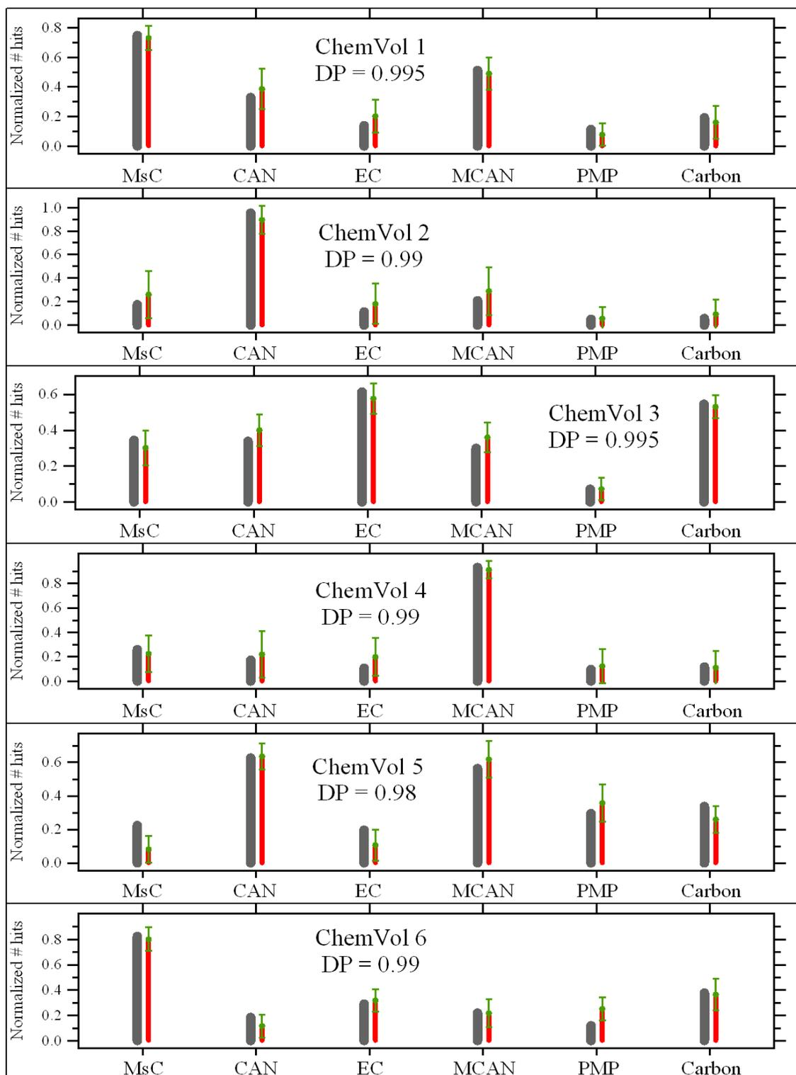
**Figure 2-3.** Side-by-side comparisons of the pre-study pooled within-cluster average class combination vectors ( $\pm 1$  standard deviation) and the ChemVol-composite vectors for the winter 2009 experiment. The dot products (DP) between the two vectors are listed.
