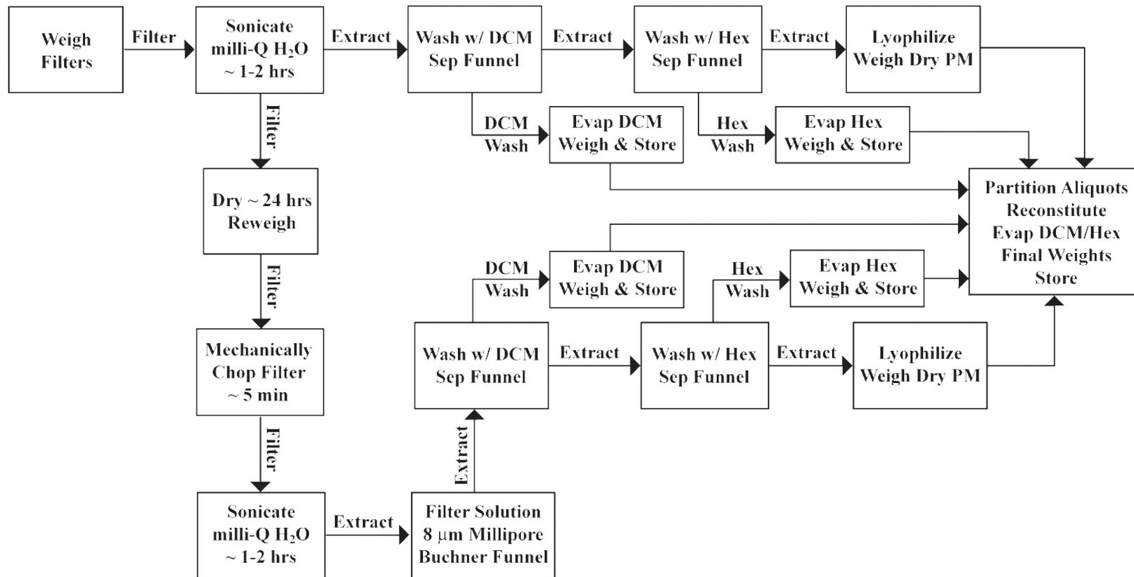
**Figure 3-2.** Flow diagram of the filter extraction and particle reconstitution process for polyurethane foam (PUF) substrates.
