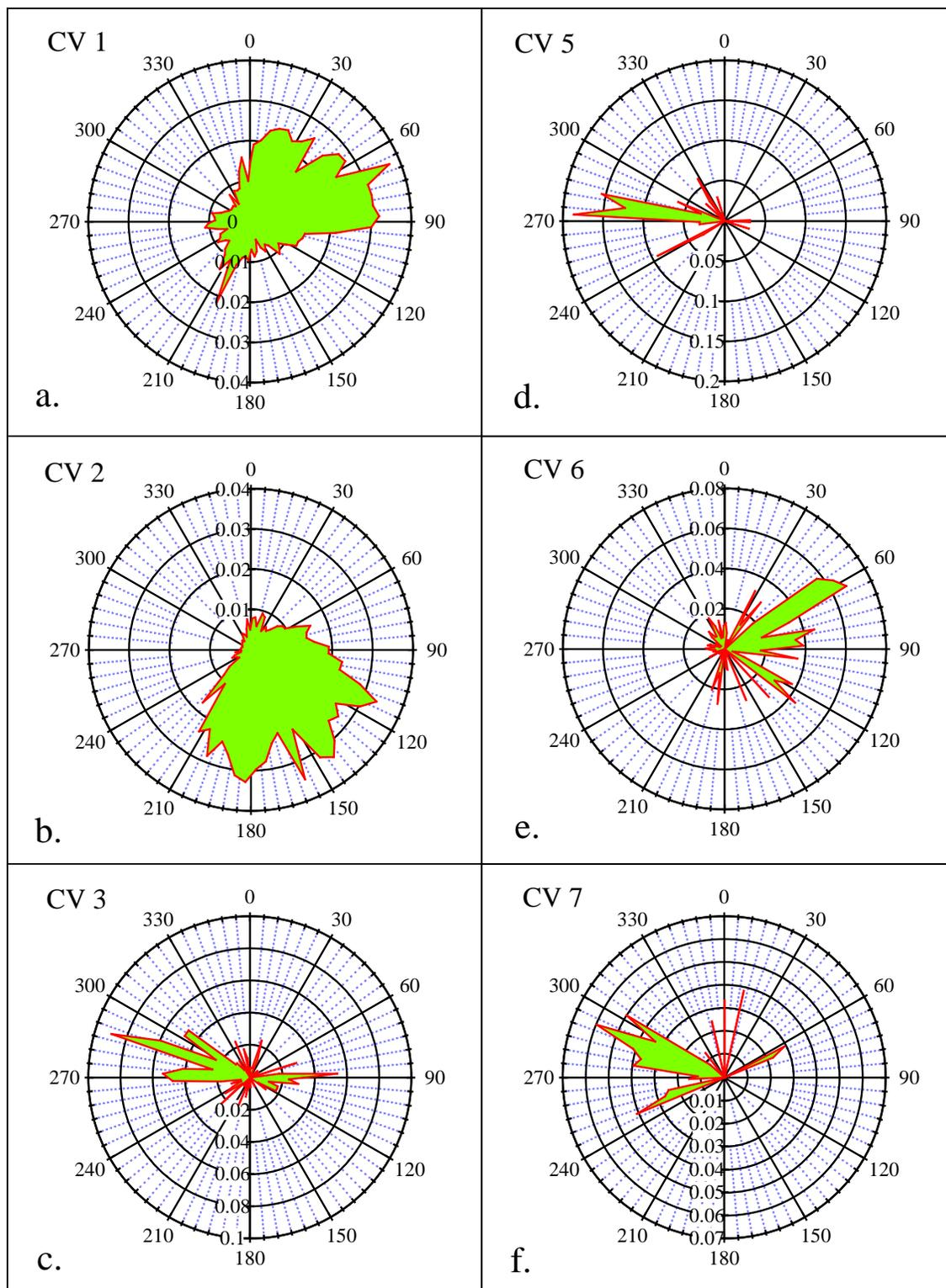
**Figure 4.3.** Wind direction frequency distributions for the source-oriented ChemVols during the summer 2008 experiment; see text for a discussion of these plots.
