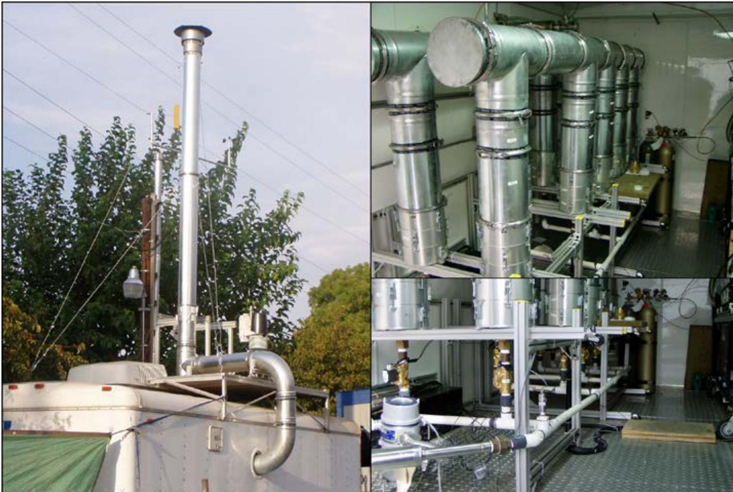
**Figure 2S-5.** Pictures of the sampling stack (left), ChemVol manifold (top) and valve manifold (bottom) inside the onsite mobile trailer; see text for discussion.
