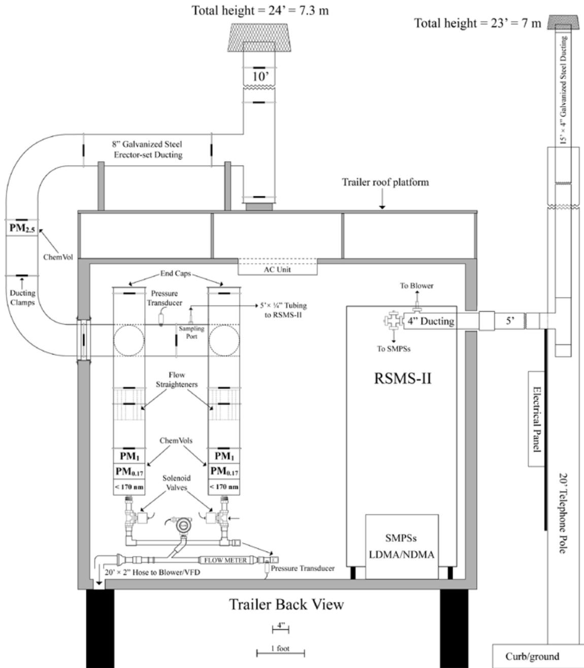
**Figure 2S-4.** A schematic of the sampling train and experimental setup; see text for discussion.
