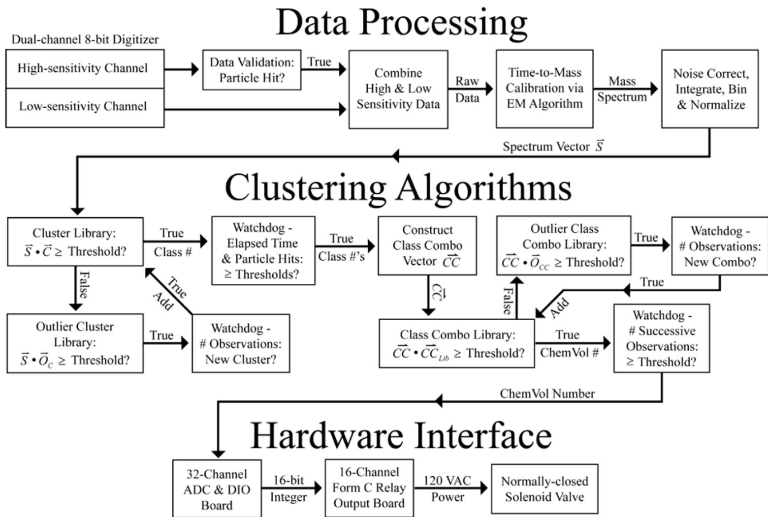
**Figure 2S-3.** Real-time data flow diagram for conditional ChemVol sampling; see text for discussion.
