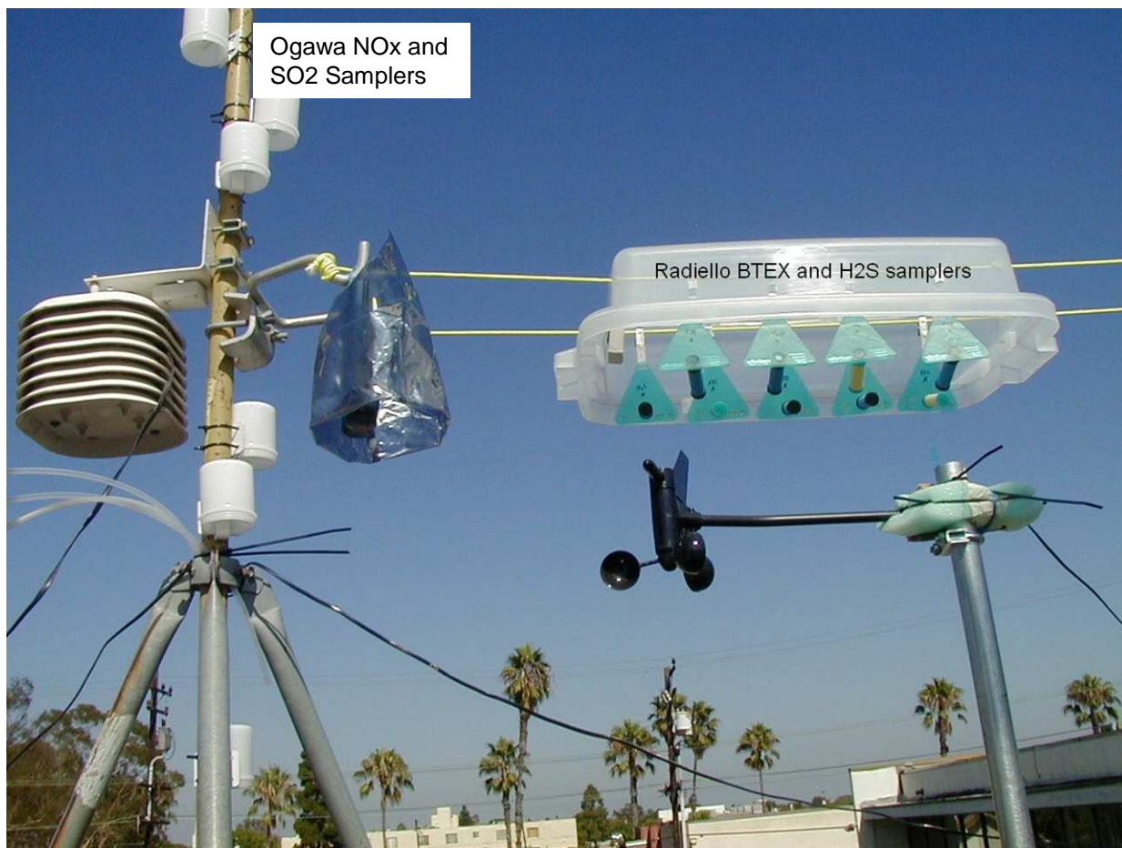
Figure 3-2. Deployment of passive samplers at the SCAQMD N. Long Beach station.
