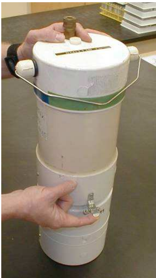
AirMetric Minivol Aerosol Sampler (20" long by 7" in diameter)
