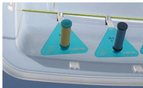
Radiello passive samplers for VOC, aldehydes and H 2 S (size of a roll of pennies)
