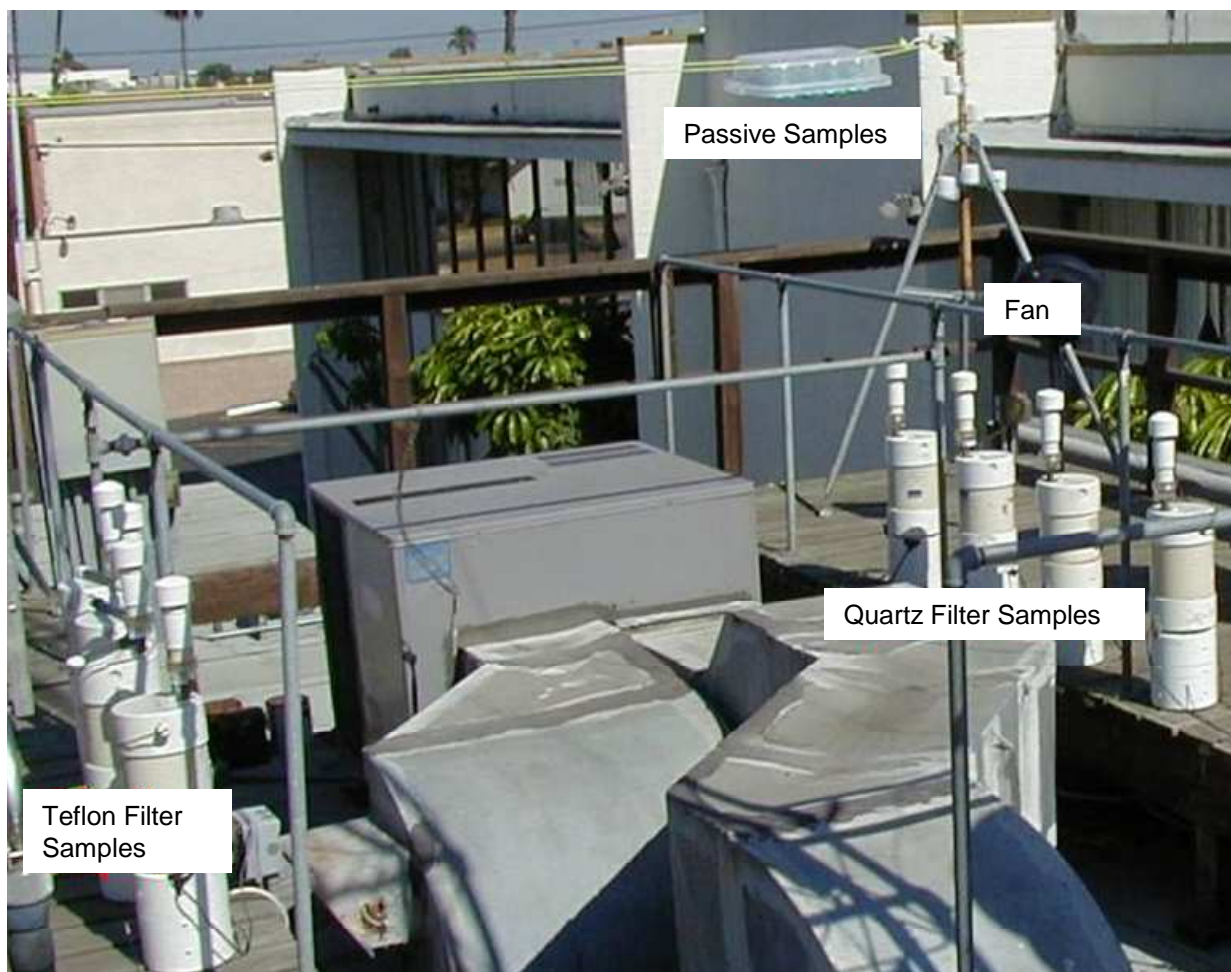
Figure 3-3. Deployment of active filter samplers (MiniVols) at the N. Long Beach station.
