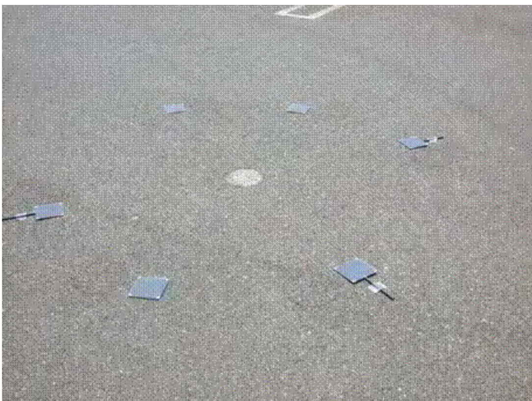
Figure 9 Views of layouts for resuspension (a) and deposition (b) experiments
