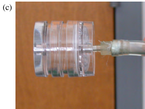
Figure 10 Views of inlet of vacuum recovery system: front (a and b); side (c)
