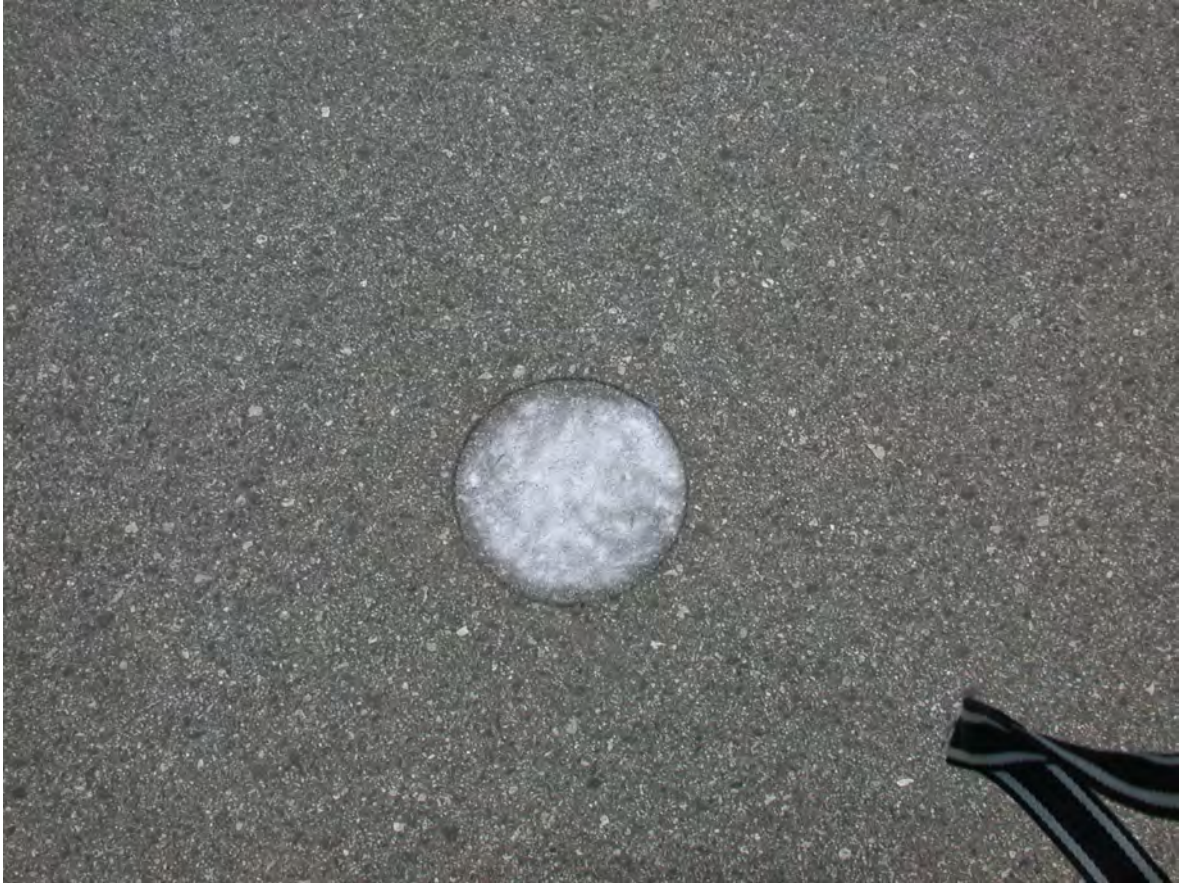
Figure18 Deployed tracer mixture on the asphalt surface showing particle agglomeration
