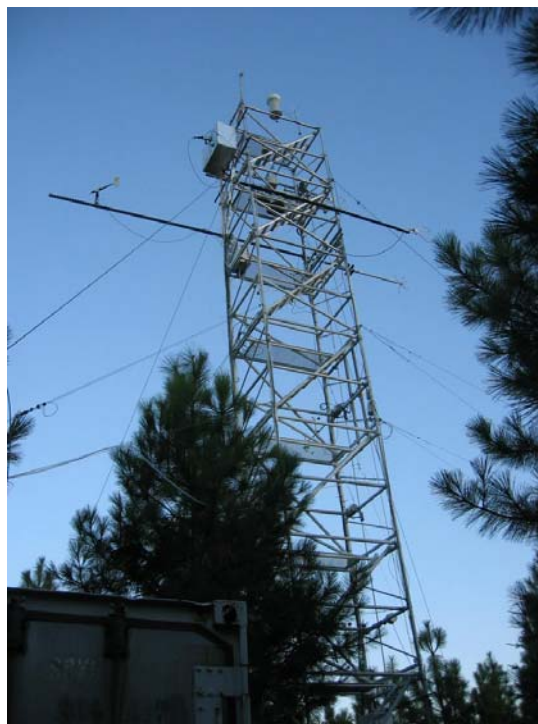
Figure 5. (Upper Left Panel) Photo showing the \text{NO}_3/\text{N}_2\text{O}_5 LIF instrument mounted on the side of the UC-BFRS tower. (Upper Right Panel) A view from the tower. Heights and species of the trees are monotonous. (Lower Panel) Photo showing a close up of the instrument (the silver shiny box to the right) on the tower.
