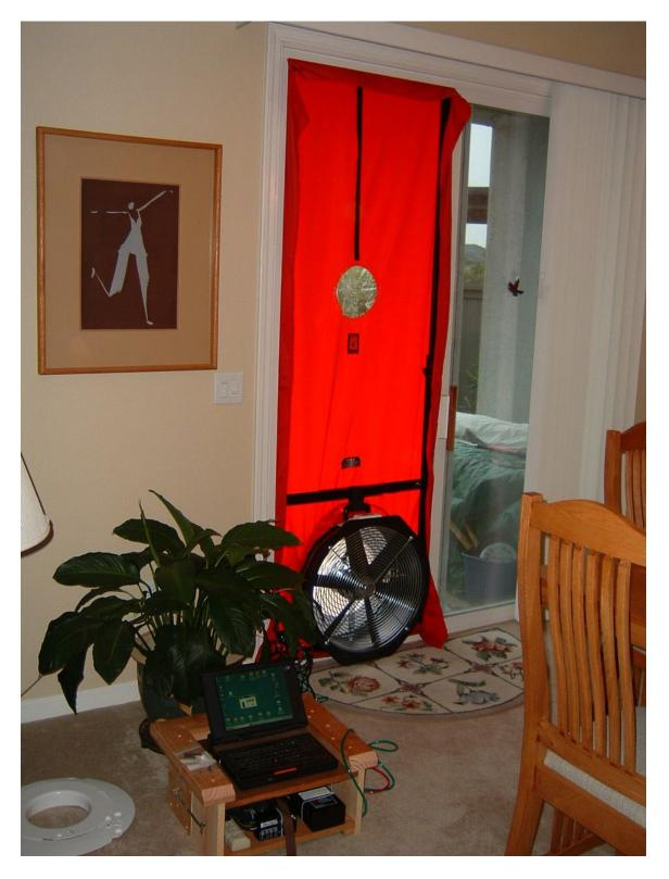
Figure 5. Pilot Home P2, Blower Door and APT installed.
