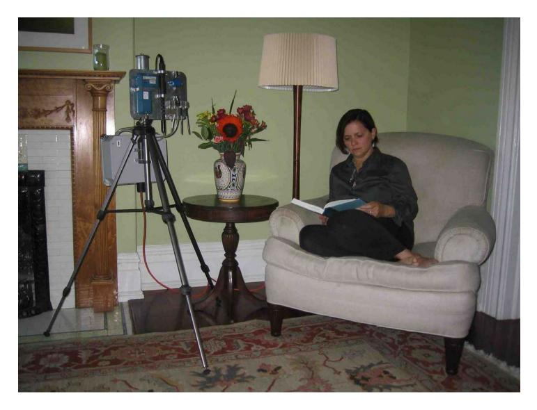
Figure 1. Quiet indoor air sampler for formaldehyde, VOCs, PM<sub>2.5</sub>, NO<sub>2</sub>, CO, CO<sub>2</sub>, temperature, and relative humidity, typically installed in a home living/dining room area for a 22–26 hour sampling period.
