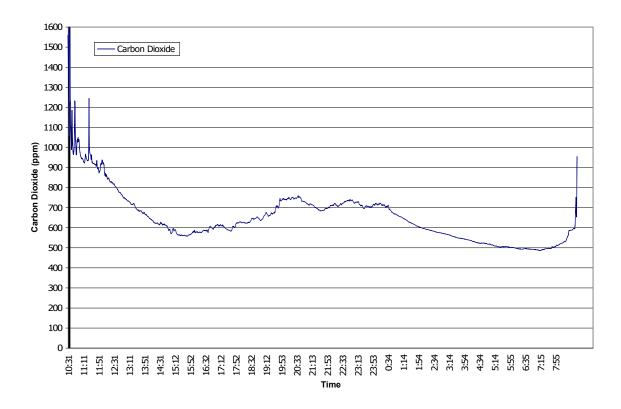
Figure 13. Concentration of carbon dioxide measured indoors at one-minute intervals in pilot home P1 between 10:19 on December 6, 2005, and 9:22 on December 7, 2005.
