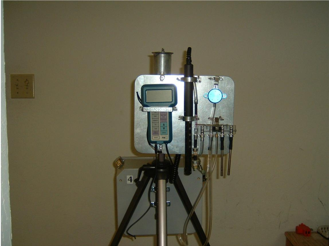
Figure 2. Close-up of air sampling rig.
