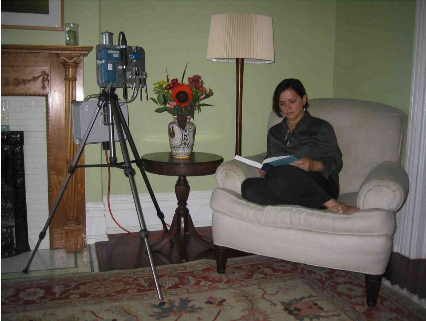
**Figure 1. Quiet indoor air sampler for formaldehyde, VOCs, PM<sub>2.5</sub>, NO<sub>2</sub>, CO, CO<sub>2</sub>, temperature, and relative humidity, typically installed in a home living/dining room area for a 22–26 hour sampling period.**
