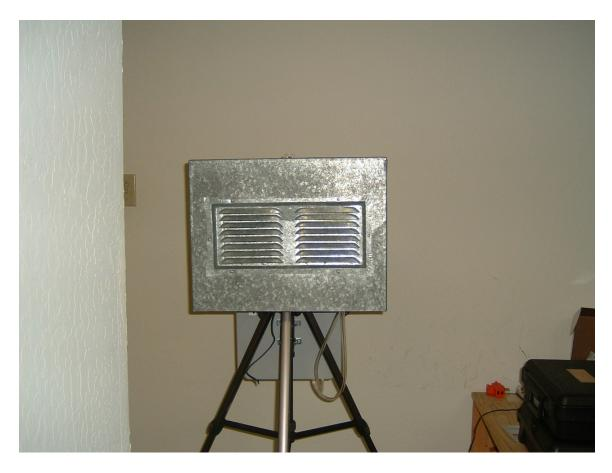
Figure 3. Close-up of air sampling rig with outdoor radiation/rain shield.
