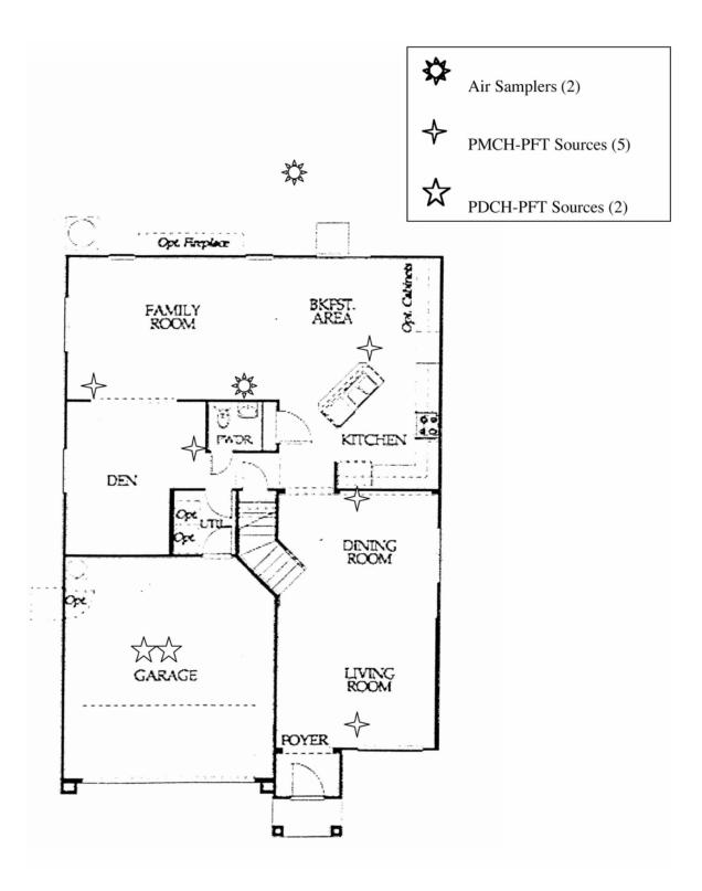
Figure 11. Floor plan of P3 first floor, depicting the locations of the air samplers and the PFT sources.
