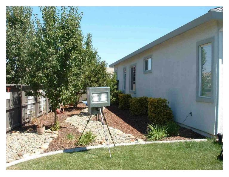
Figure 2. Outdoor air sampler for formaldehyde, VOCs,  $PM_{2.5}$ ,  $NO_2$ , CO,  $CO_2$ , temperature, and relative humidity, with outdoor radiation/rain shield.
