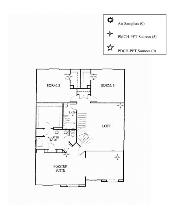
Figure 12. Floor plan of P3 second floor, depicting the locations of the PFT sources.
