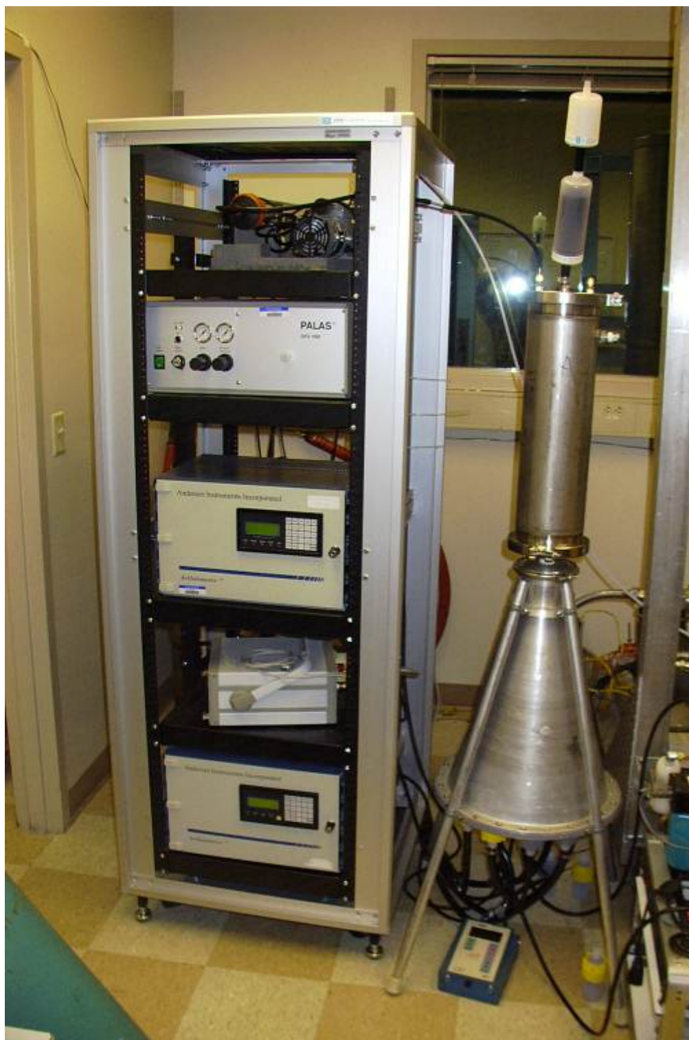
Figure 3-11. PALAS electric arc soot generator experimental setup showing the instrument rack, the miniature dilution/residence chamber with dilution air through an in-line HEPA filter and activated charcoal, and the conical sampling manifold.
