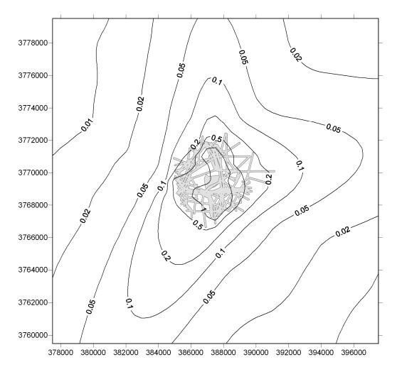
Figure 4: UP LATC Railyard off-site sources and railyard with modeled annual average concentrations from off-site sources in  $\mu g/m^3$
