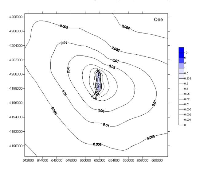
Figure 9. AERMOD's Simulated Diesel PM Concentrations (Due to On-site and Off-site Diesel PM Emissions)
