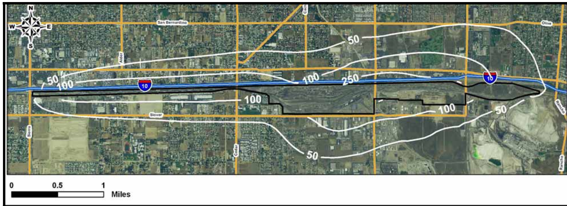
Figure V-1: Estimated Near-Source Cancer Risks (chances per million people) from the UP Colton Railyard
