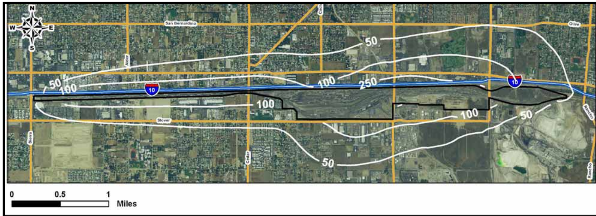
Figure II-3: Estimated Near-Source Cancer Risks (chances per million people) from the UP Colton Railyard
