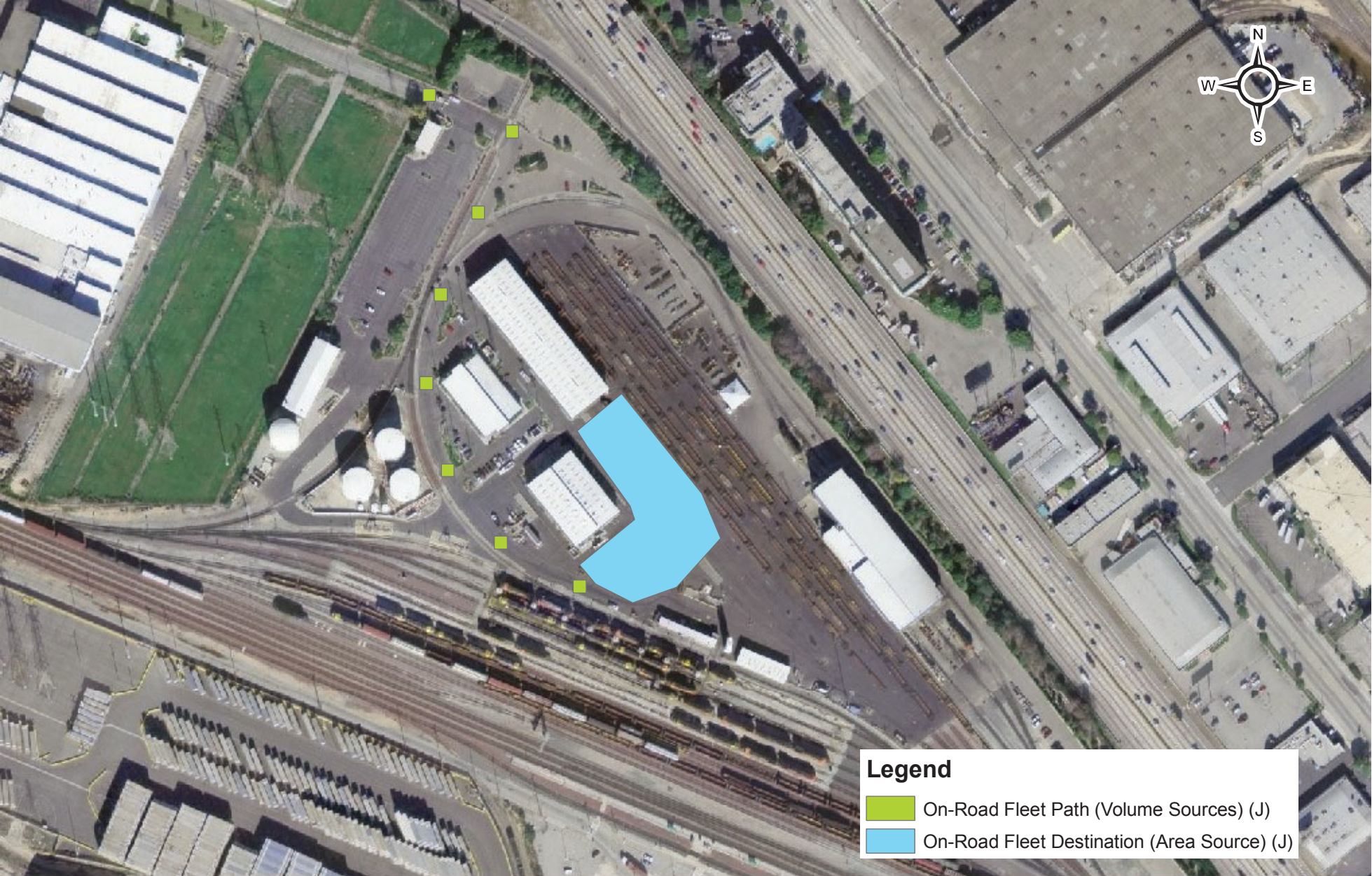
Figure 4-4b: Locations of Modeled On-Road Fleet Sources (Travel Route 2) BNSF Commerce Mechanical Rail Yard Commerce, California
