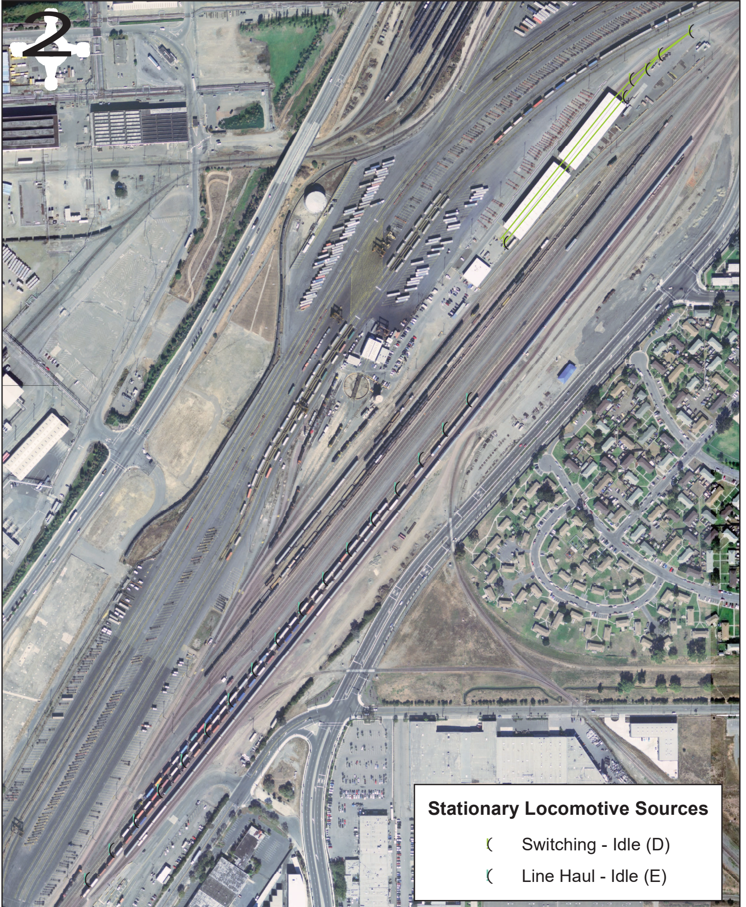
Figure 4-1b: Locations of Modeled Stationary Locomotive Sources - Switching and Line Haul BNSF Richmond Rail Yard Richmond, California
