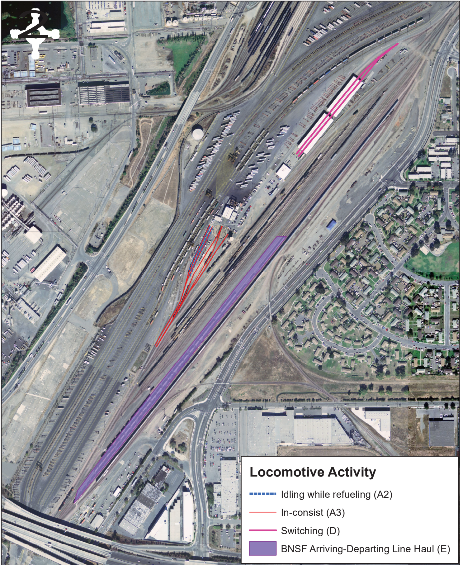
Figure 2-3a: Stationary Locomotive Activities BNSF Richmond Rail Yard Richmond, California
