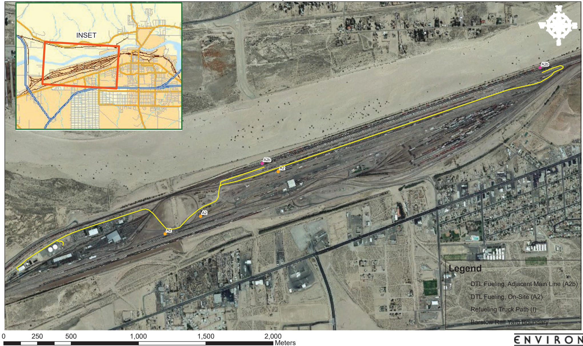
Figure 2-7: Stationary Locomotive Refueling at DTL Areas and On-Site Refueling Truck Activities BNSF Barstow Rail Yard Barstow, California
