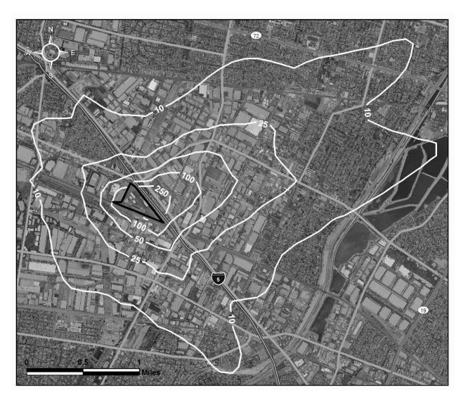
**Figure V-1** Estimated potential cancer risks (chances per million) associated with onsite diesel PM emissions at the BNSF Sheila Mechanical Railyard facility (based on 80th percentile breathing rate and 70-year exposure).
