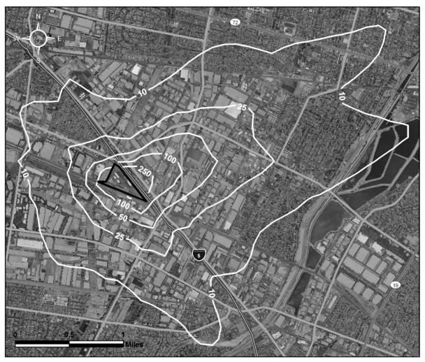
**Figure II-3** Estimated potential cancer risks (chances per million) associated with the diesel PM emissions from the BNSF Sheila Mechanical Railyard (based on 80th percentile breathing rate and 70-year exposure).
