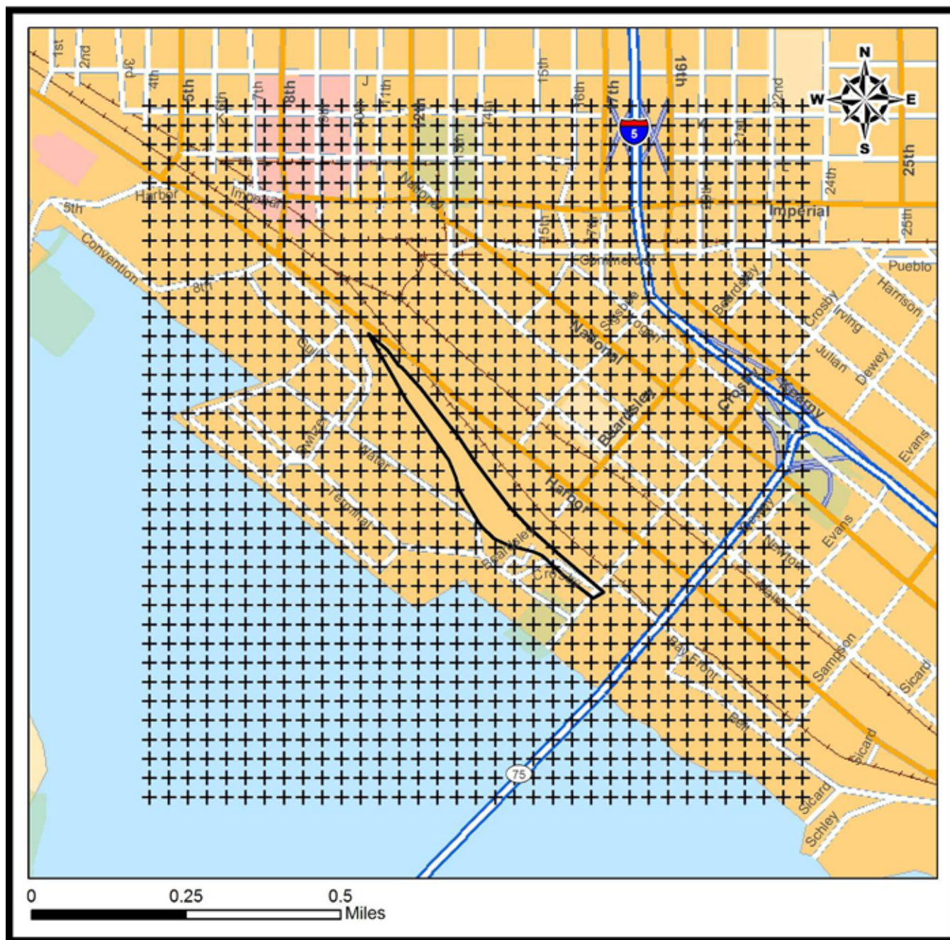
Figure IV-6: Fine Grid Receptor Network Air Dispersion Modeling for BNSF San Diego Railyard
