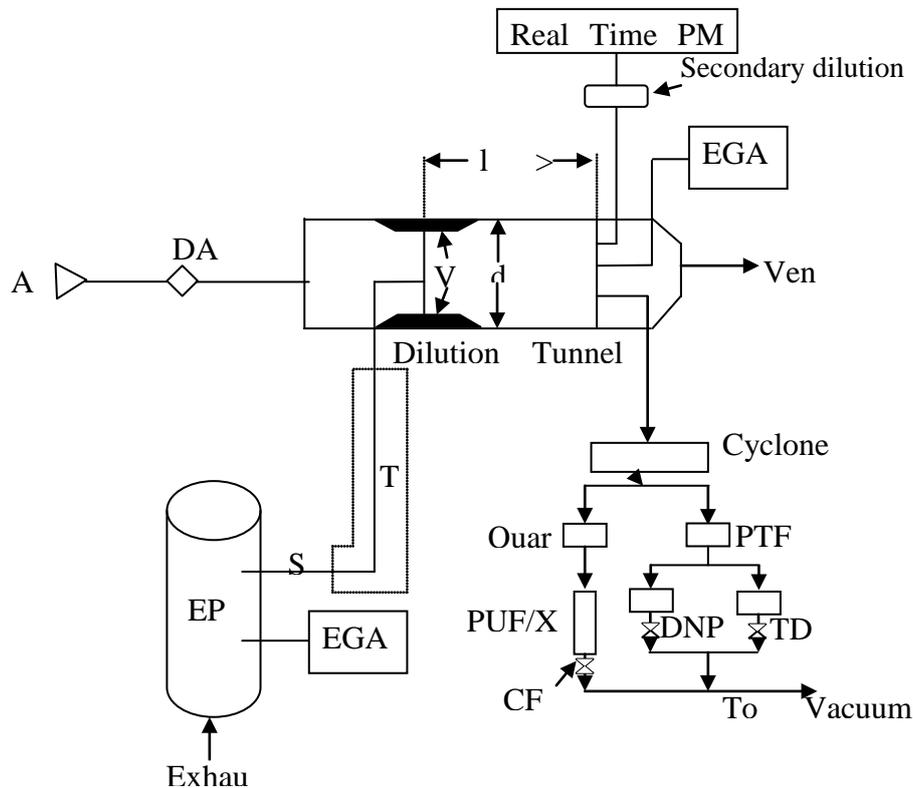
**Figure 10-4 Partial Flow Dilution System with Added Separation Stages for Sampling both Regulated and Non-regulated Gaseous and PM Emissions**
