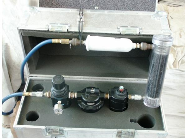
**Figure 10-2 Field Processing Unit for Purifying Dilution Air in Carrying Case**
