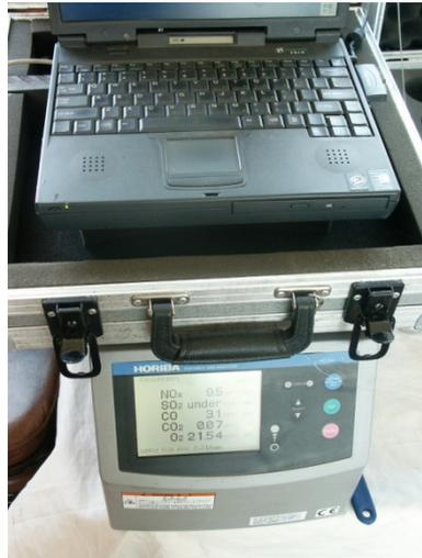
Figure 10-3 Setup Showing Gas Analyzer with Computer for Continuous Data Logging
