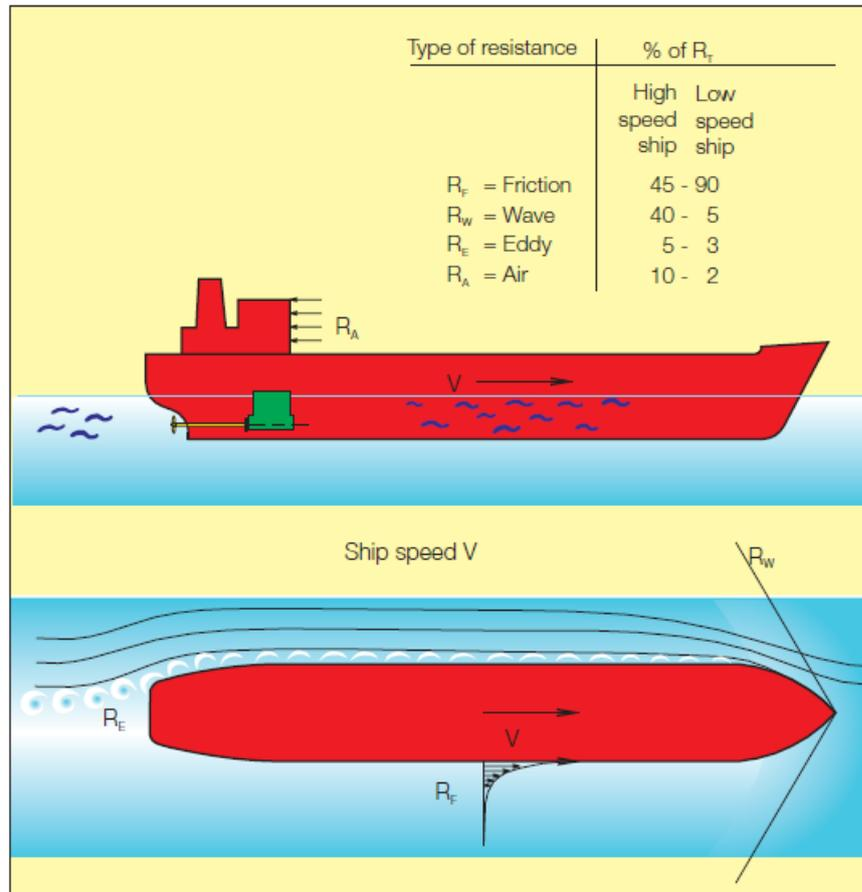
**Figure 13-1 Total Ship Towing Resistance  $R_T = R_F + R_W + R_E + R_A$**
