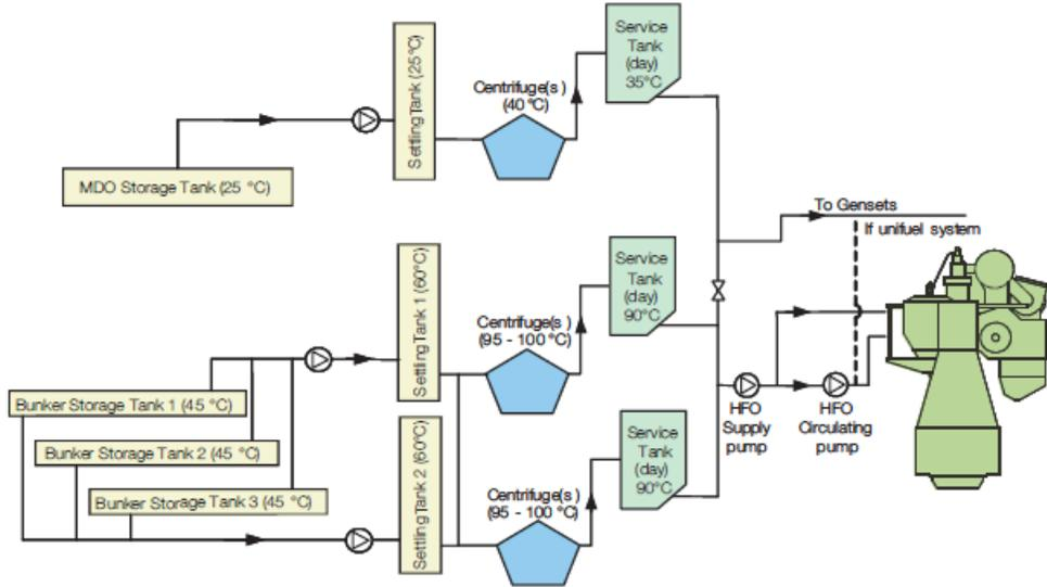
Figure 6-5 One MDO Settling Tank and Two Sets of HFO Settling and Service Tanks<sup>6</sup>
