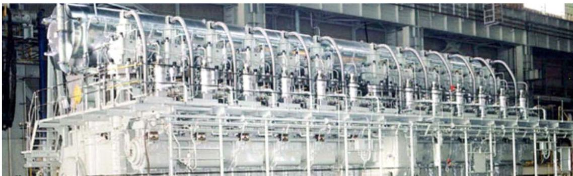
**Figure 4-1 MAN Picture showing Model MAN B&W 11K98ME7**
