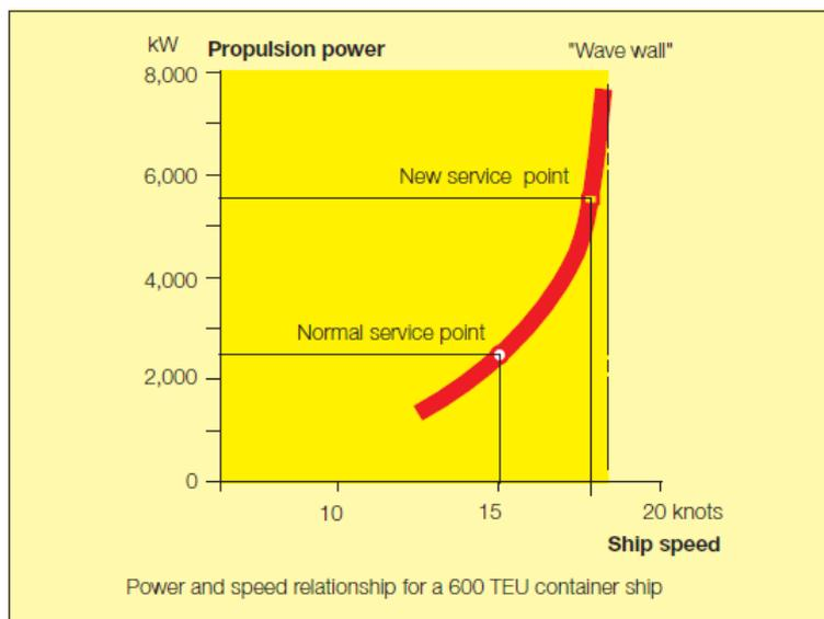
Figure 13-2 The “Wave Wall” Ship Speed Barrier
