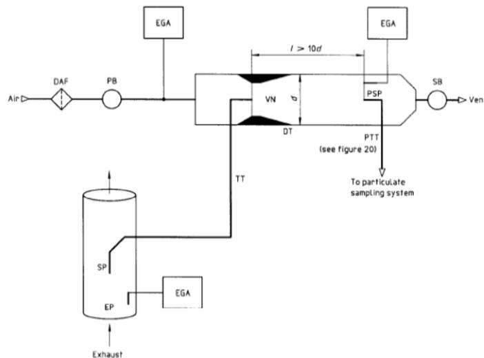
**Figure 10-1 Partial Flow Dilution System with Single Venturi, Concentration Measurement and Fractional Sampling**
