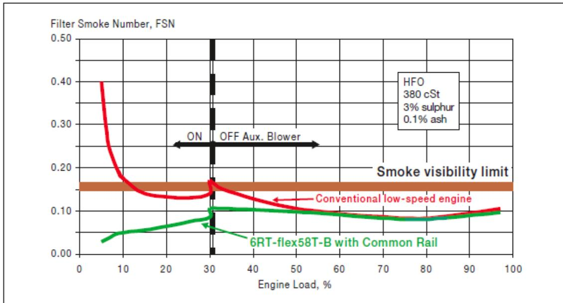
Figure 6-3 Example of Engine Design with Auxiliary Blower
