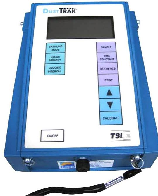
Figure 10-5 Picture of TSI Dust Trak
