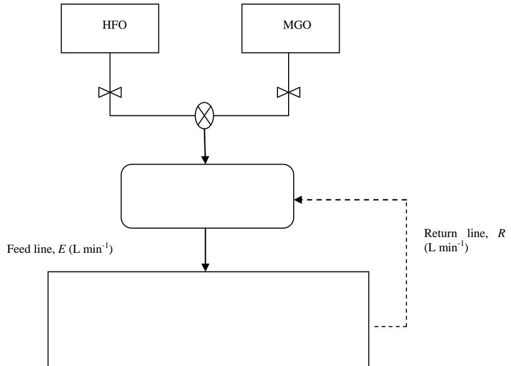
**Figure 6-6 Fuel flow system for marine diesel engine**
