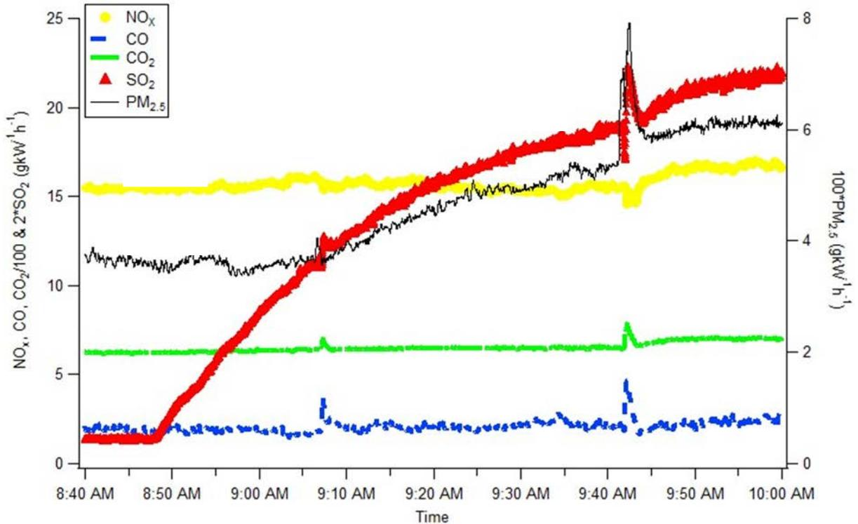
**Figure 5-3 Fuel Switching from MGO to HFO**
