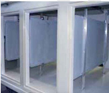
Figure III.B-2: Partition Mount (Johnson Truck Bodies)
