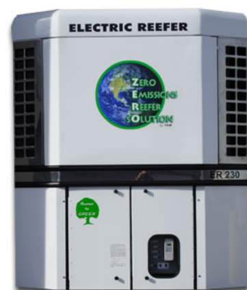
Figure III.A-1: Converted All-Electric TR
