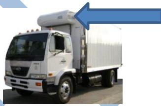
Figure 20 to the right shows an all-electric plug-in / battery Auragen transport refrigerator on a mid-sized truck.
