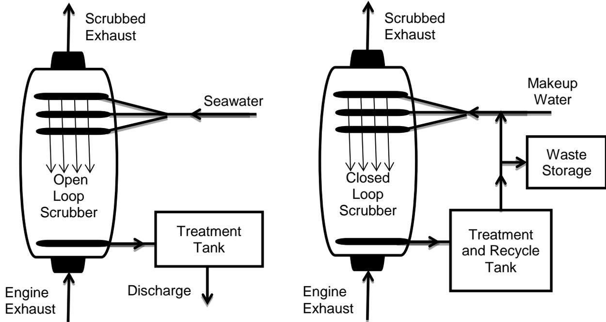
Hybrid systems use seawater, but have the capability of recycling their water while operating for a limited time in sensitive inland waterways. These are the most flexible systems and are able to operate in all ECA zones, but they are also the most complex.
