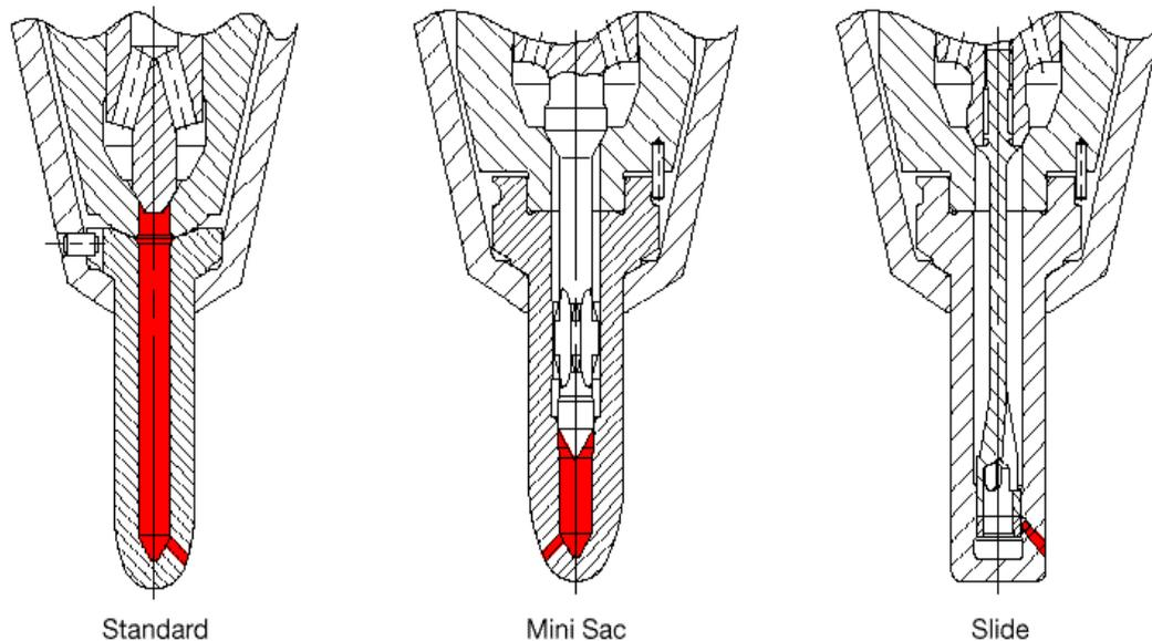
The potential challenge with fuel injectors (both conventional and slide valves) is that they can be designed for lower NO<sub>x</sub> (with the tradeoff of slightly higher fuel consumption) or for maximum fuel efficiency (and higher NO<sub>x</sub>).
