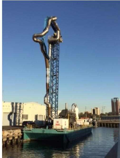
The barge based exhaust cleanup systems captures the vessel's exhaust directly from the exhaust stack, using long, flexible ducting to transfer the exhaust smoke back to the barge to be cleaned. Flexible ducting is brought by crane to the vessel's stack. The current systems operate under a strong vacuum to reduce any leakage of air from the
