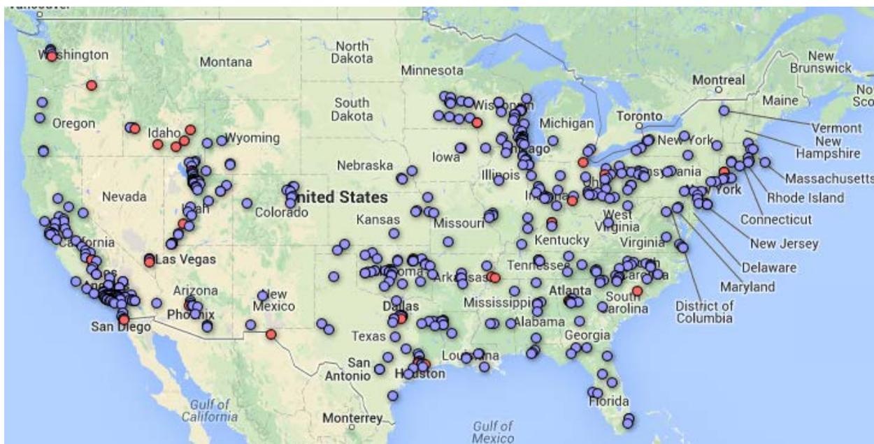
Red dots represent LNG stations, and blue dots represent CNG stations
