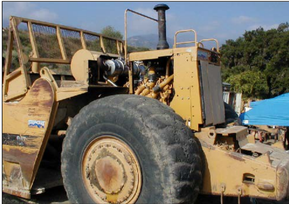
657E scraper with a 2007 Caterpillar C15 On-Road Engine
