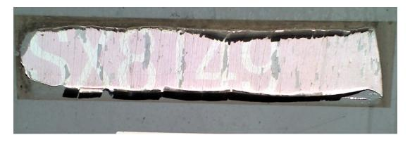
To clarify, the regulation requires that the EIN be maintained in a manner that retains its legibility for the entire life of the vehicle. This requires that if an EIN label becomes illegible, it must be replaced; it does not require that the original label must last the life of the vehicle.
