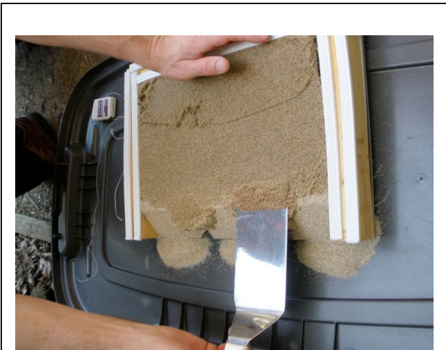
Figure 3. Post-infiltration excavation of dual plumes of CARB#2 and Soy B20 biodiesel showing homogeneous plume structure between walls indicating absence of wall effects on infiltration.
