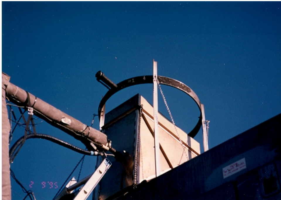
FIGURE 4. SwRI SMOKEMETER INSTALLED ON A LOCOMOTIVE
