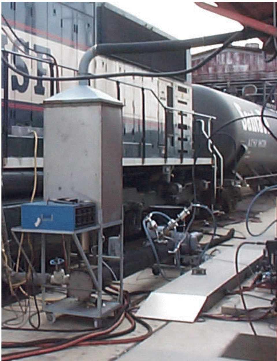
FIGURE 1. EMISSIONS TEST SETUP USED FOR SAMPLING PARTICULATE
