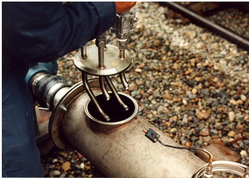
FIGURE 3. PARTICULATE SAMPLE PROBES LOCATED WITHIN DILUTION TUNNEL
