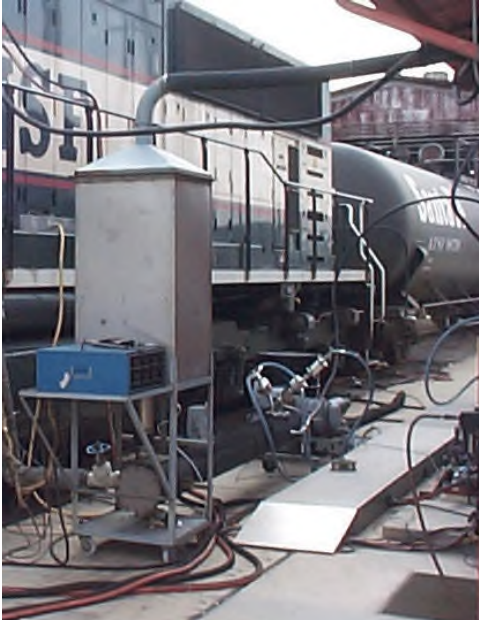
FIGURE 1. EMISSIONS TEST SETUP USED FOR SAMPLING PARTICULATE
