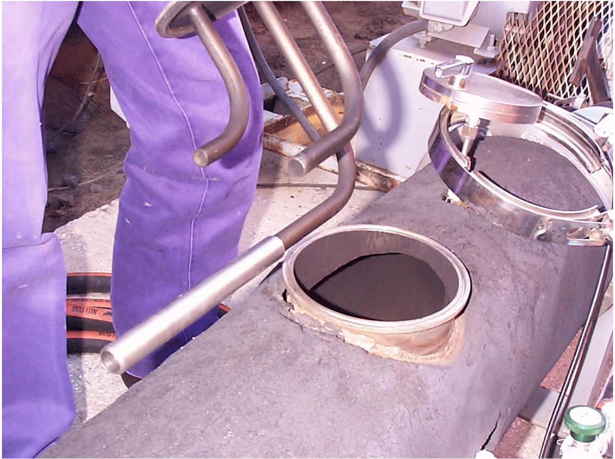
FIGURE 2. ISOKINETIC PARTICULATE SAMPLE PROBE USED WITHIN DILUTION TUNNEL FOR PARTICLE SIZING MEASUREMENTS
