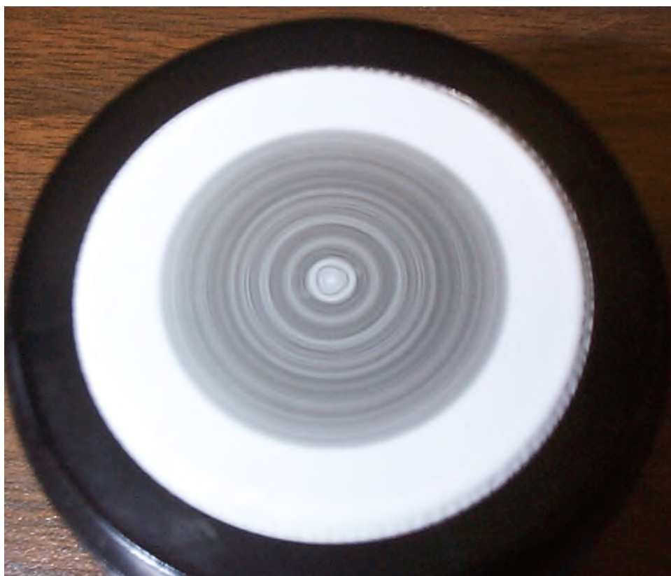
FIGURE 4. PARTICULATE COLLECTED ON ONE OF THE IMPACTION PLATES OF A MOUDI STAGE
