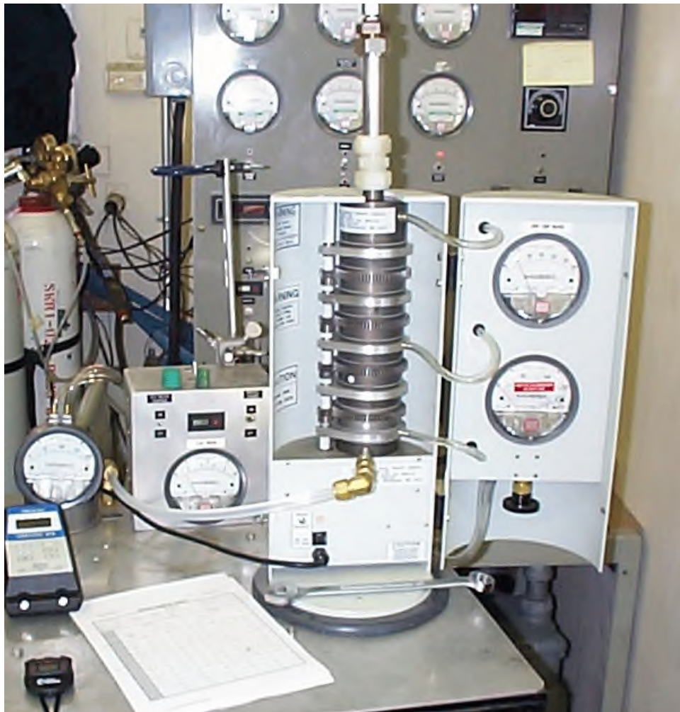
FIGURE 3. MOUDI PARTICLE SIZE SYSTEM USED AT LOCOMOTIVE TEST CENTER
