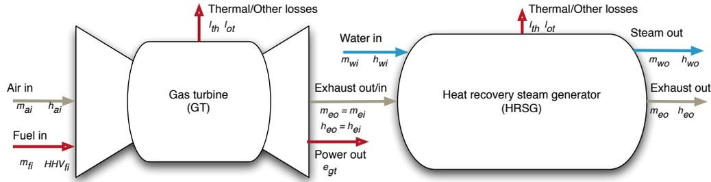
Figure 5.3: Gas turbine plus heat recovery steam generator model. Mass flows represented by  $m$  and energy flows represented by fuel lower heating value (LHV), electric power out ( $e$ ) and enthalpy of gases ( $h$ ).
