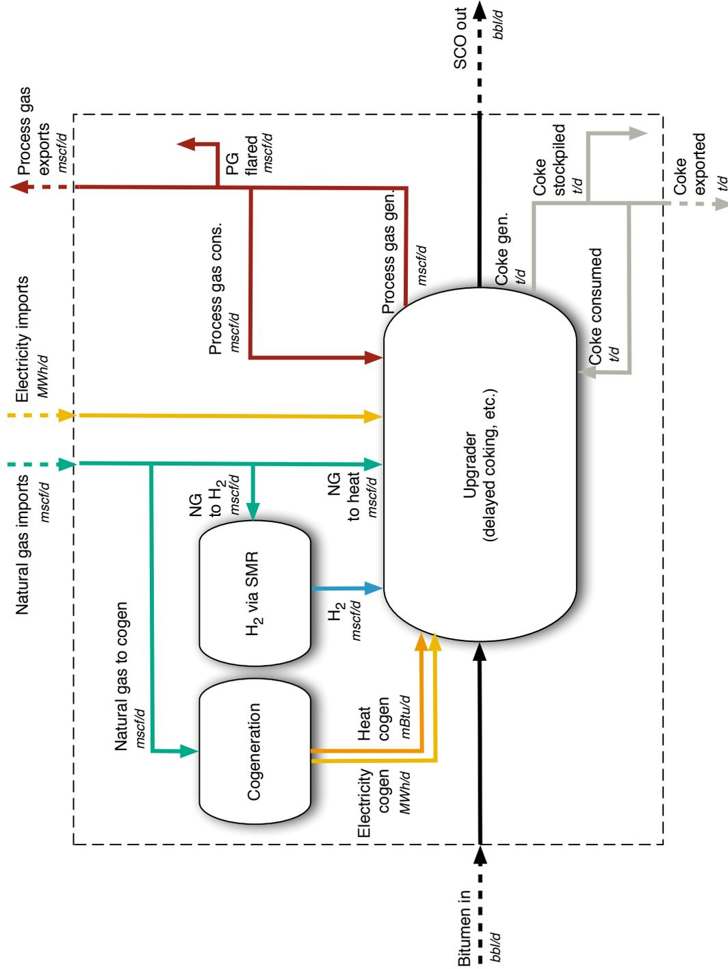
Figure 4.25: Process flow diagram for OPGEE upgrading module
