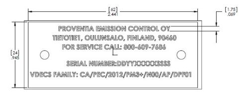
Note: This label is attached to both the filter and the engine.
