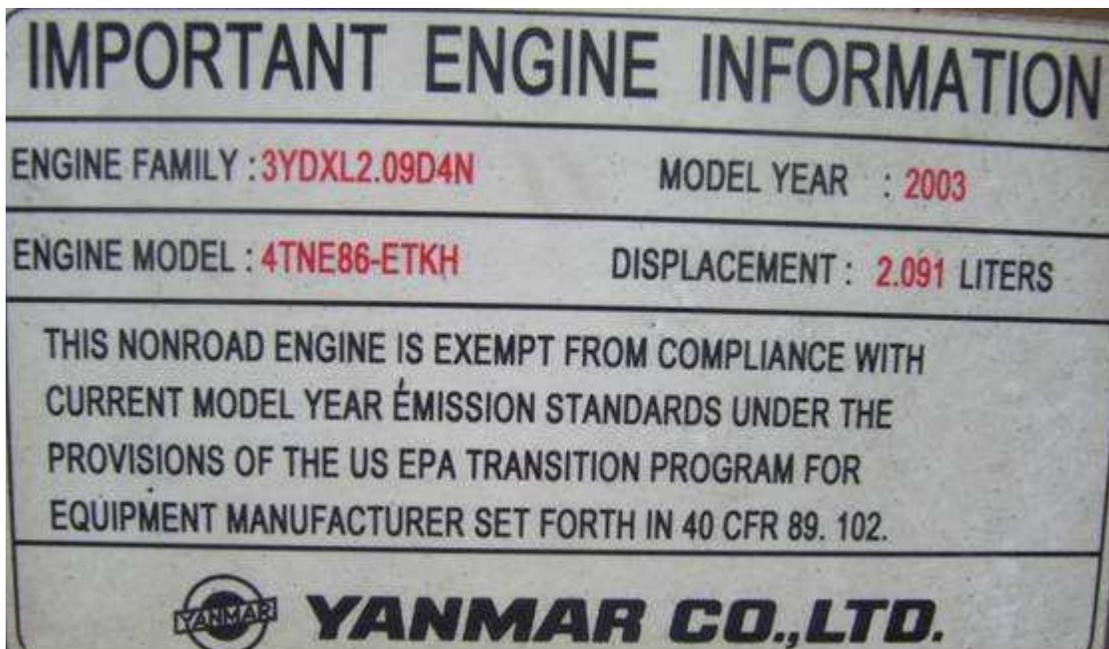
Figure-1 Yanmar 2005 Manufactured Engine Labeled as 2003 TP EM
