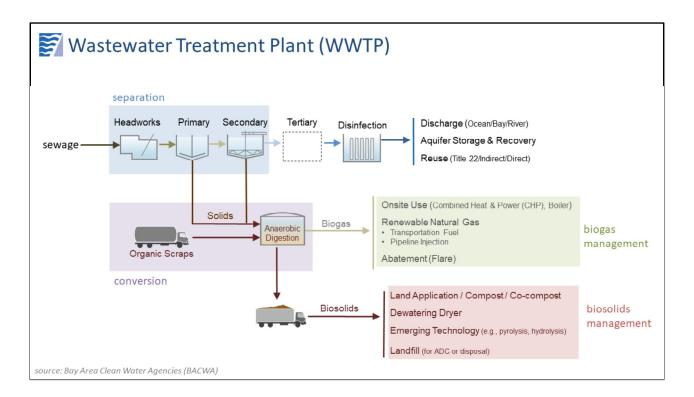
This slides generalizes the design of a wastewater treatment plant.
