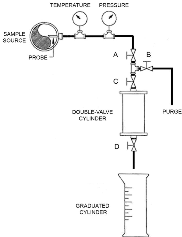
**8.9** Collect liquid sample: Slowly open valve D to allow a slow displacement of the non-reactive displacement liquid at a rate not to exceed 60 milliliters per minute to prevent the sample liquid from flashing. Continue until approximately 70 percent of the displacement liquid is measured in the graduated cylinder. Then close valves D and C.
