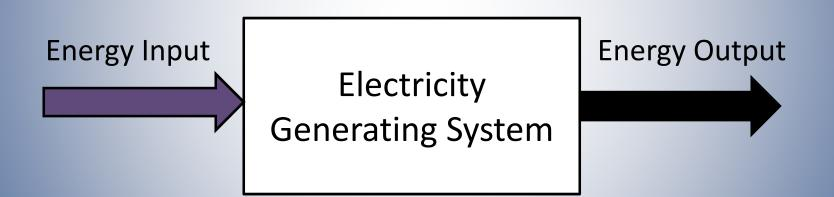
The difference between energy input and energy output is the energy that is wasted (e.g., heat released to the atmosphere, formation of air pollutants, vented steam, mechanical friction).
