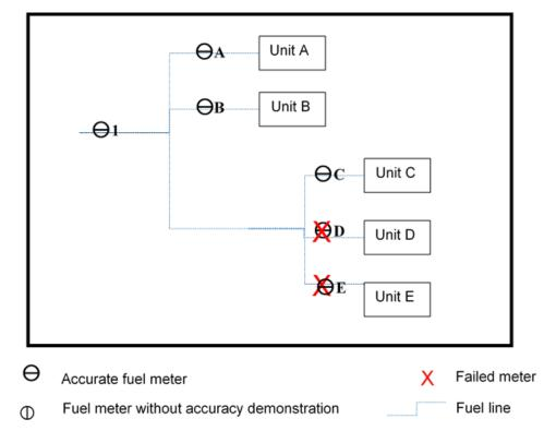
Example 7: Accurate Facility-Level Meter and Failed Unit Meters
