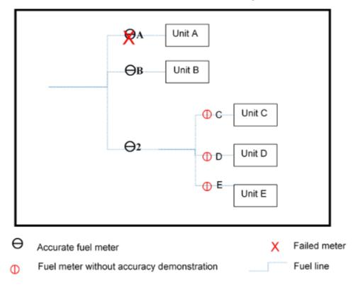
Example 3: Unit with Failed Meter and No Alternate Upstream Data
