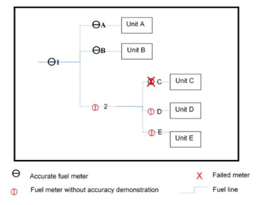
Example 5: Accurate Facility-Level Meter and Failed and Unknown Downstream Meters
