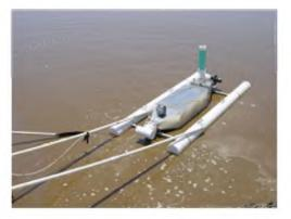
A floating wind tunnel for measuring the emissions from lagoons
