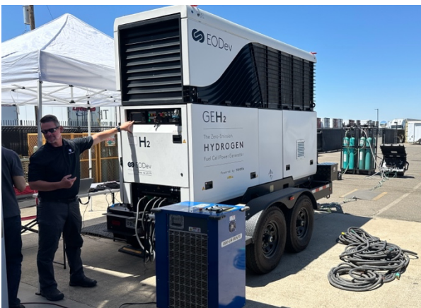
Figure 2. H2FC Generator and Load Bank Installed at the Test Site
