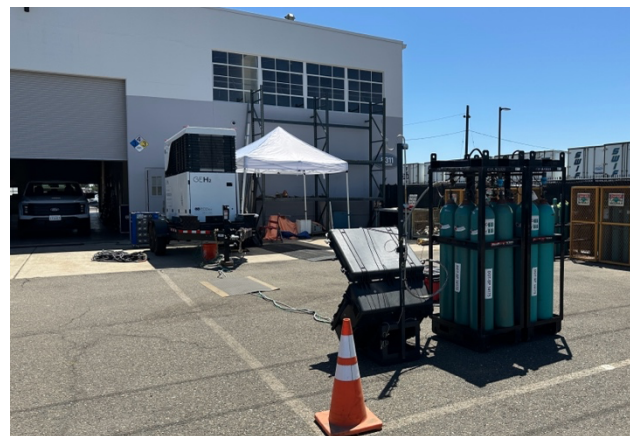
Figure 3. Hydrogen Storage Cylinders and Pressure Regulation System Connected to the H2FC Generator
