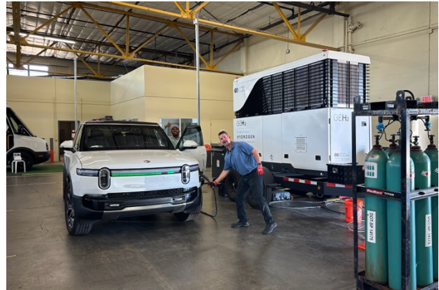
Figure 7. H2FC generator demonstration powering an electric vehicle
