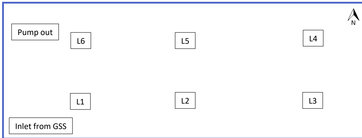
Figure 3.2 Dairy 1 pond schematic for sampling locations during quarterly sampling.
