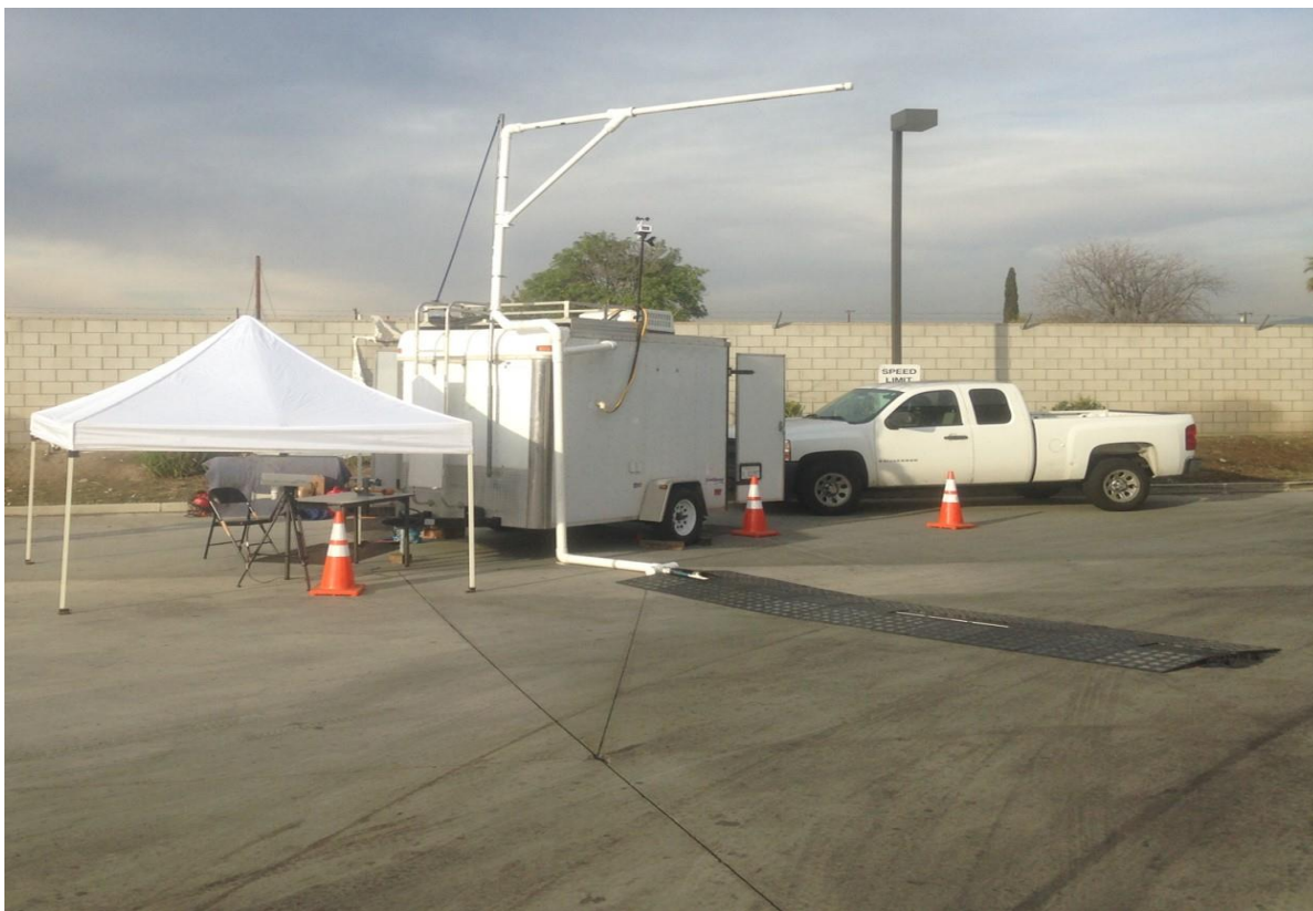
Figure 3-5 Picture of PEAQS setup at the J&R facility
