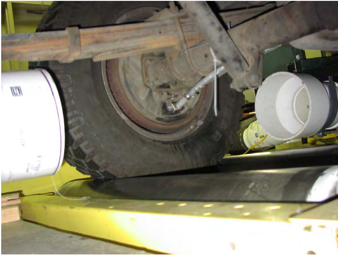
Figure 2.5.2 Photograph of the split dilution tunnel sections mounted on the vehicle undercarriage, showing the free air space between the upstream (left) and downstream (right) tunnel sections.
