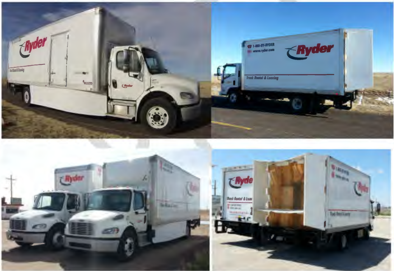
Figure 1. Vehicles with Aerodynamic Devices Installed. Class 6 (left), Class 4 (right), Coastdown Vehicles (top), On-Road Test and Control Vehicles (bottom)
