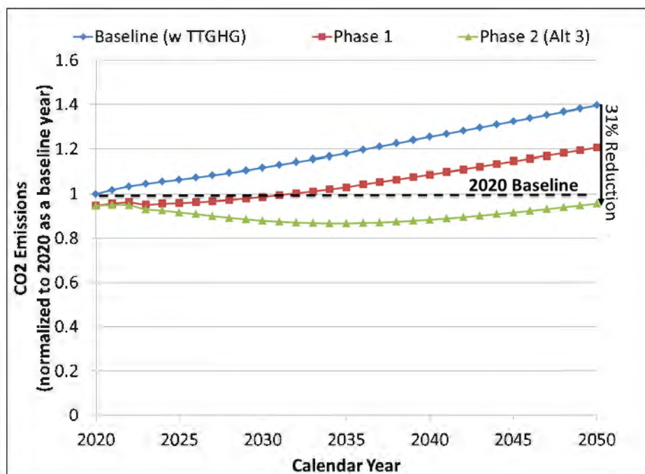
Figure 1: Statewide On-Road GHG Emissions (Normalized to 2020 as a Baseline year) from Phase 2 Regulated Vehicles: without Regulation (Baseline including CARB Tractor-Trailer Regulation), with the Phase 1 Regulation, and with the Alternative 3 of Phase 2 Regulation
