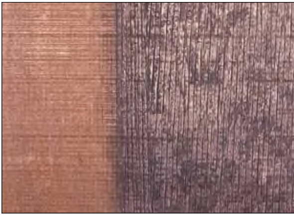
Figure 16–18. Front view of exterior grade of plywood siding after 10 years of exposure. The right-hand portion was exposed to the weather, whereas the left-hand side was covered with a board to give a board-and-batten appearance.
