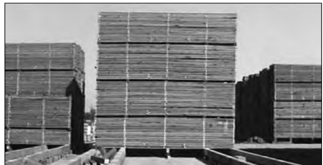
Figure 14–7. A sanitary, well-drained air-drying yard.
