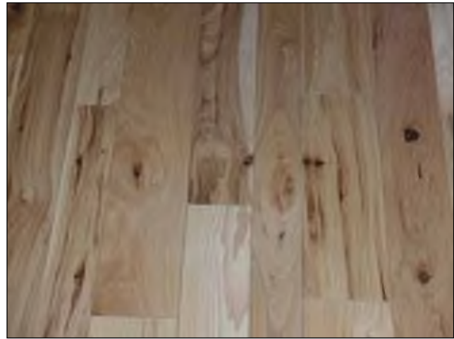
Figure 16–31. Number 2 grade of hickory finished to accentuate the beauty of the various colors, knots, and grain pattern of this species.
