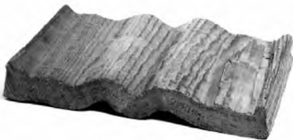
Figure 13-10. Severe collapse in western redcedar.
