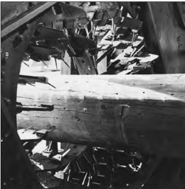
Figure 15-4. Deep incising permits better penetration of preservative.
