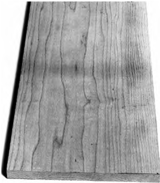
Figure 13–17. Sticker stain in sapwood of sugar maple after planing.
