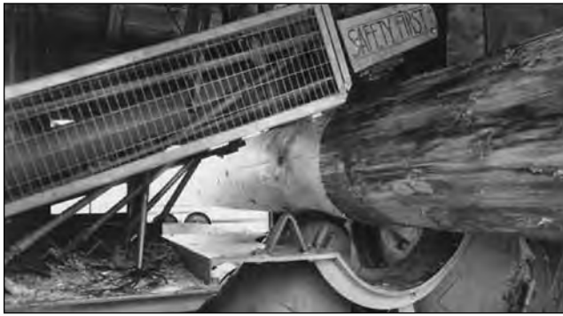
Figure 15-3. Machine peeling of poles. The outer bark has been removed by hand, and the inner bark is being peeled by machine. Frequently, all the bark is removed by machine.
