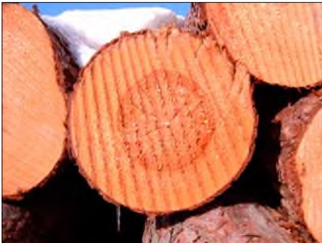
Figure 13-9. End checking in red pine logs.
