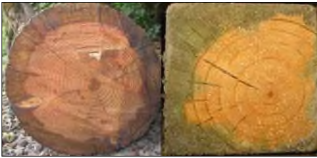
Figure 15–2. During pressure treatment, preservative typically penetrates only the sapwood. Round members have a uniform treated sapwood shell, but sawn members may have less penetration on one or more faces.
