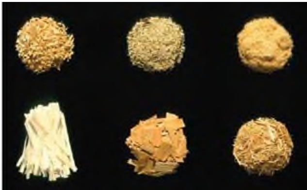
Figure 11–5. Common wood elements used in wood-based composites from top left, clockwise: shavings, sawdust, fiber, large particles, wafers, and strands.
