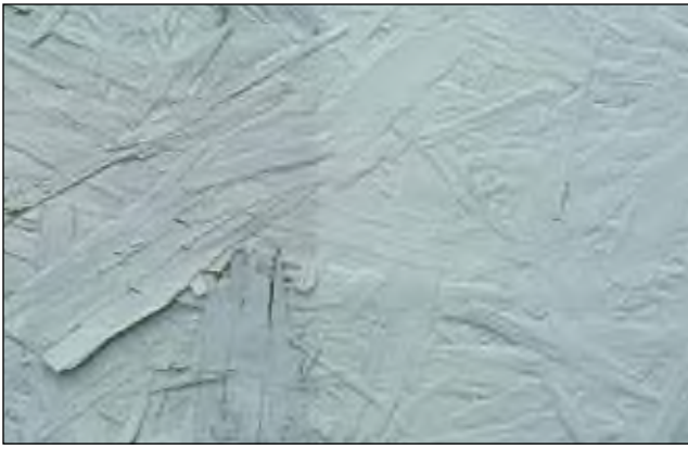
Figure 16–11. Absorption of water causes differential dimensional change of surface flakes to give an uneven surface (telegraphing).
