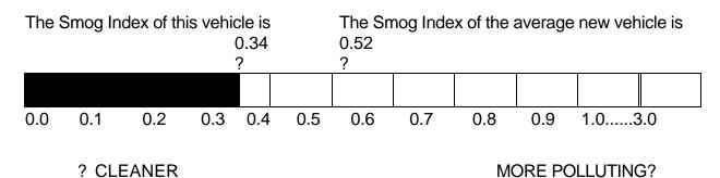
Note: The Smog Index (SI) indicates the relative level of smog-forming pollutants emitted by the vehicle. The lower the SI, the lower the vehicle's emissions.
